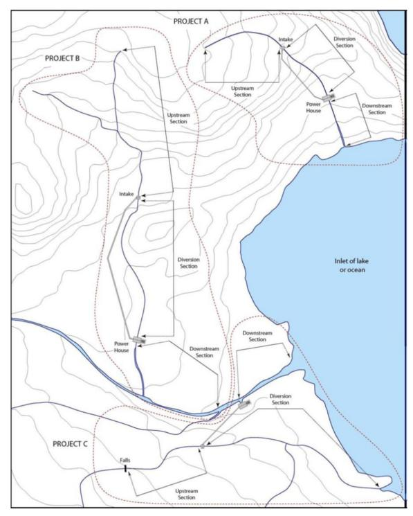
Figure 2.Examples of upstream, diversion, and downstream sections for three hypothetical hydroelectric projects (taken from Lewis et al. 2004).
