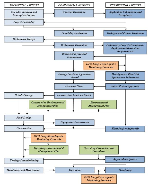
Figure 1. Typical Project Development Sequence for an Independent Power Producer (modified from Province of British Columbia 2010).
