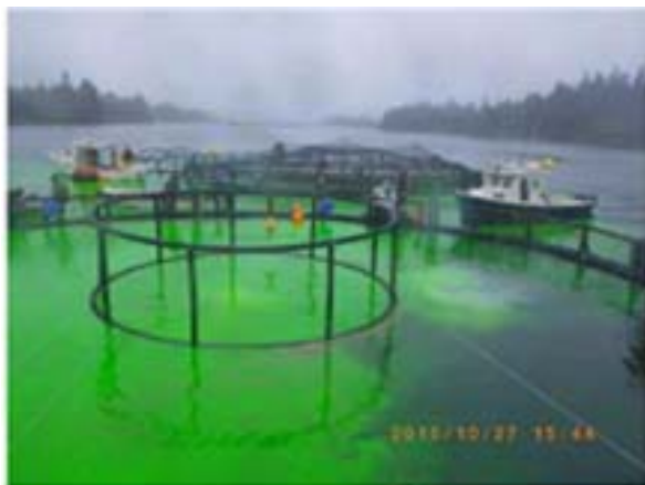
Green fluorescein dye, used to measure therapeutic transport and dispersal, being released from an Atlantic salmon net pen following an anti-sea lice tarp bath treatment. (courtesy of Fred Page, DFO, St. Andrews Biological Station)
