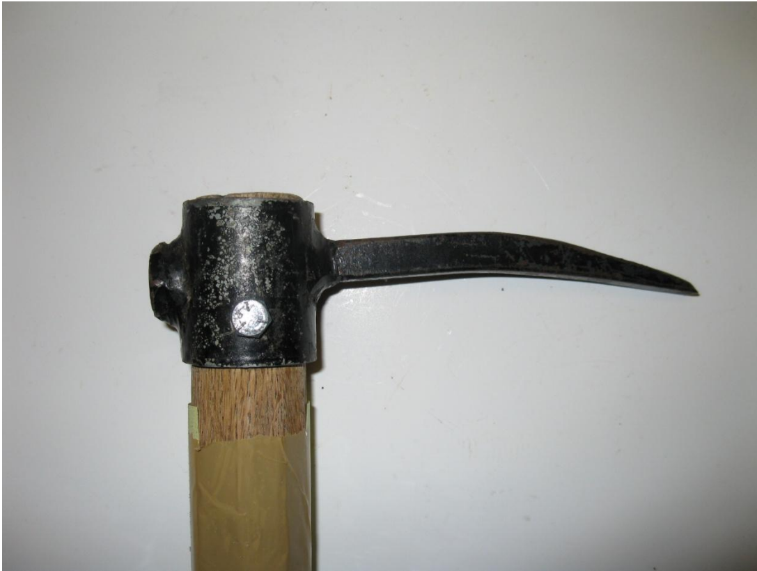
Figure 1. Canadian hakapik used to measure forces required to effectively crush the skull of harp and grey seal beaters, March 2010.
