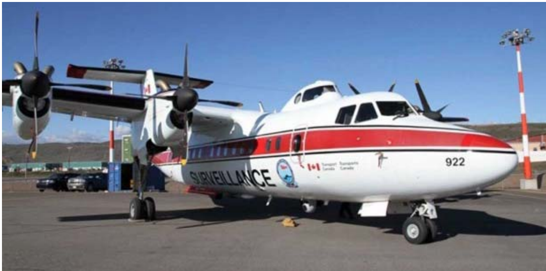
Figure 3: Dash-7 Ice Reconnaissance and Oil Pollution Surveillance Aircraft (Photo courtesy of CIS)
