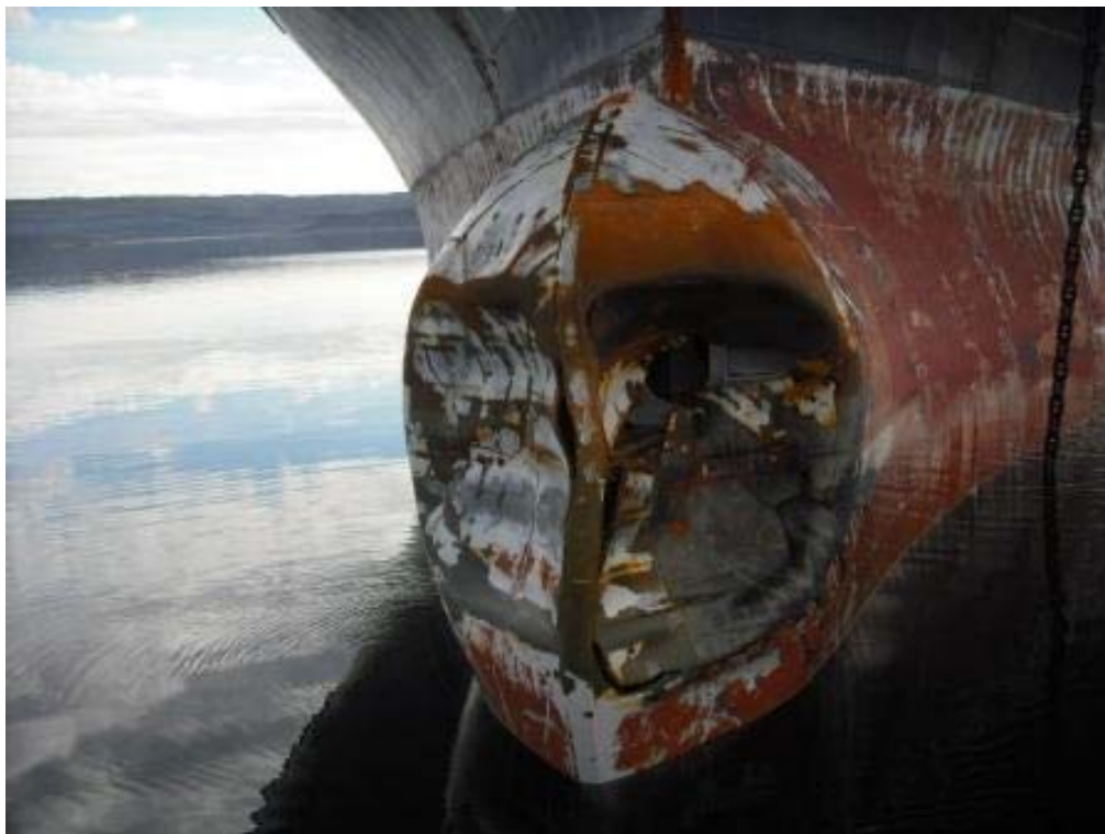
Figure 43 Bulbous bow of a cargo vessel with a Lloyd's 100 A1 Ice Class 1A damaged in ice enroute Iqaluit, Nunavut, in July
