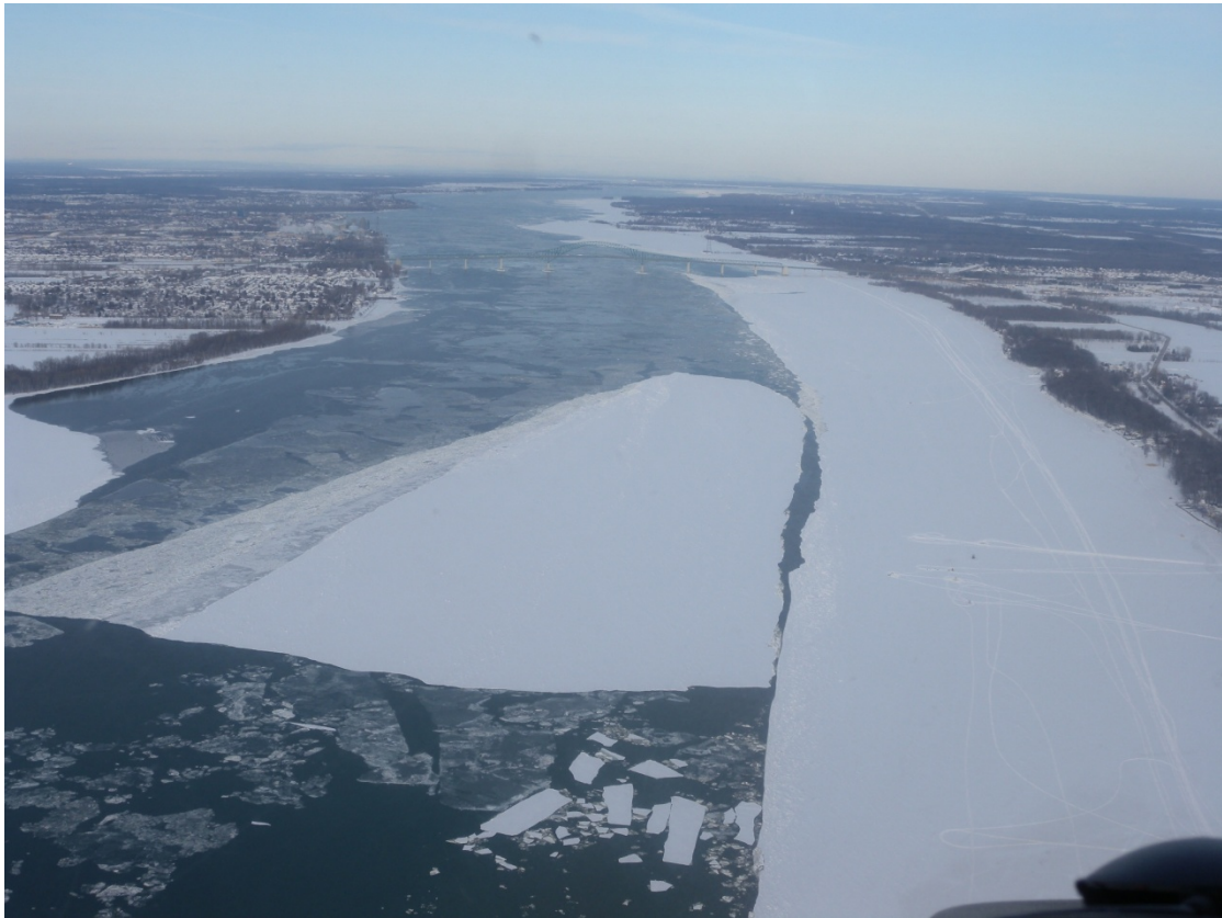
Figure 29: The ship channel can be easily blocked if ice is dislodged from the banks
