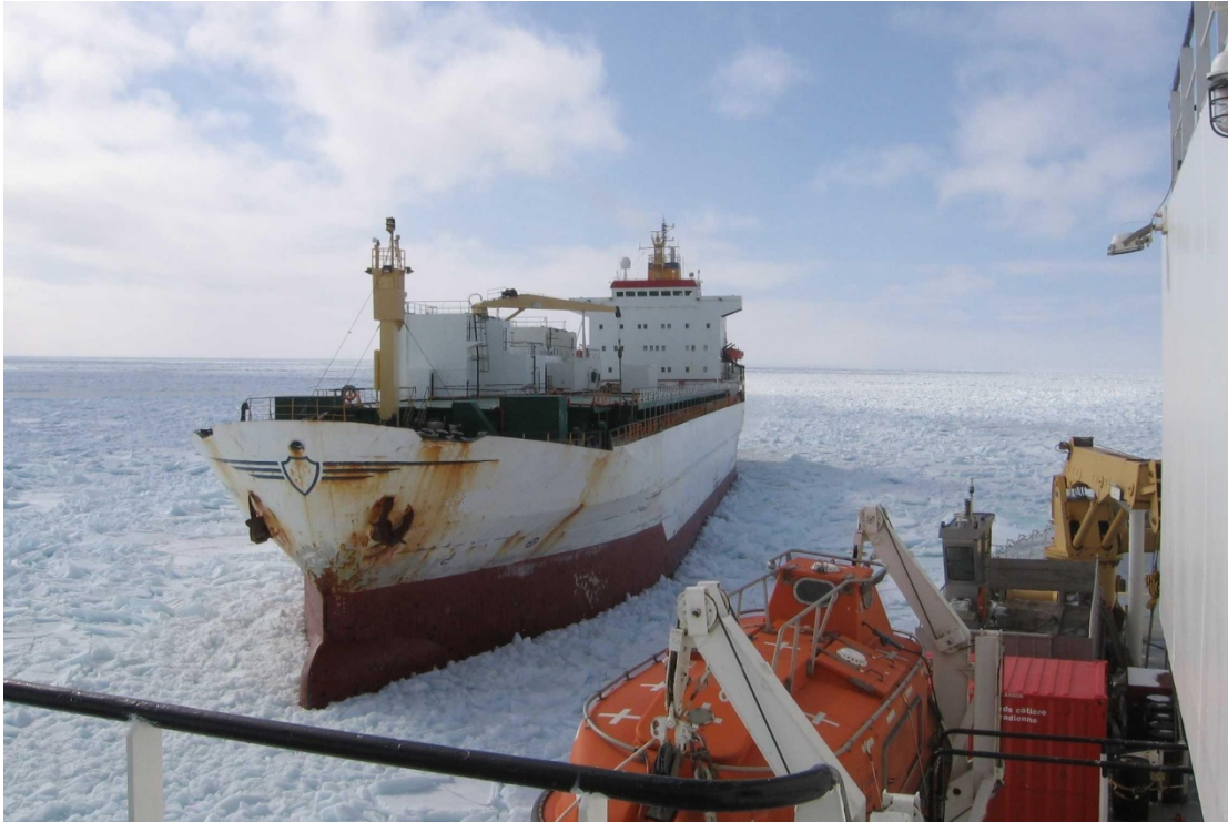
Figure 48: Icebreaker backing alongside vessel to free it from the ice
