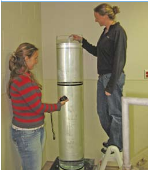
Figure 1. Settling rate experiments using a sedimentation column.
