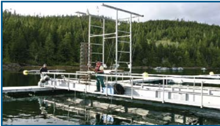
Figure 3. The shellfish component of the Kyuquot SEAfoods SEAfood System™, specifically showing the SEA-Tram and its gantry on the new floatation structure.
