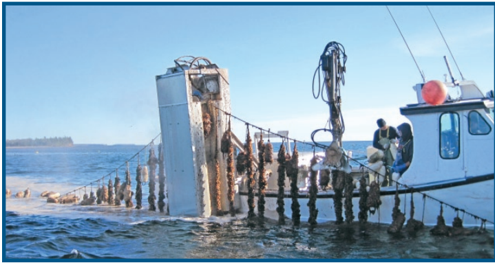
Figure 3. Technology developed by mussel producers in eastern PEI to reduce the level of C. intestinalis fouling on mussel socks. The technology uses high-pressure spray nozzles to remove tunicates from the mussel socks.
