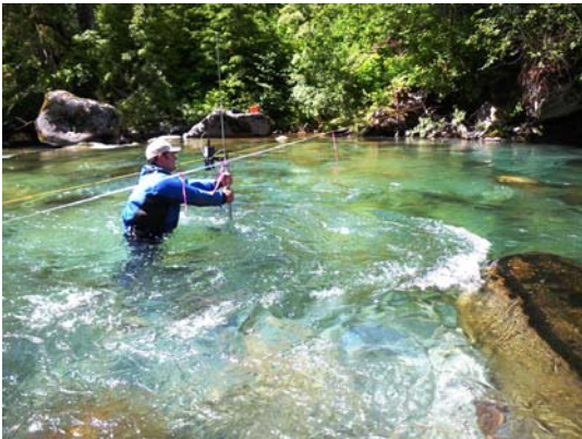
Figure 1: Measuring flow. Photo with permission of Adam Lewis, Ecofish Research Ltd.
