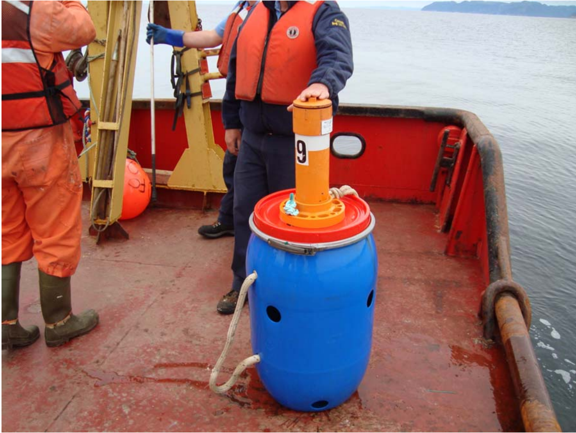
Figure 2. Convertible Accurate Surface Tracker (CAST) drifter out of the water. The central orange cylinder contains the electronics package including the GPS receiver and transmitter.
