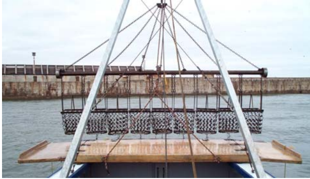
Figure 5: Digby-type dredge commonly used in the Gulf Region showing tow bar and steel ring buckets.
