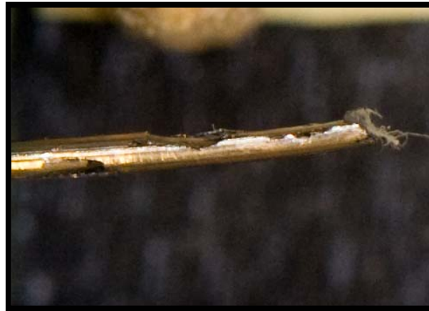
Figure 8. Photograph of a corroded nickel pin after 18 weeks of immersion in seawater.
