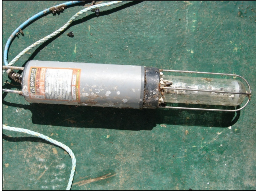
Figure 1. Aquastar aquaculture machine systems, submersible photoperiod lighting 800 W 220 V-50 HZ bulb type: halogen metal with Ignitor 11 cm diameter 100 cm length, bulb life: 12,000 h, colour yield - 90 CRI colour temperature: 6500 degrees K glass type: boro silicate. 5 mm). Six of these were used in a 70 m polar circle cage holding Atlantic cod in the Bay of Fundy, near Back Bay, New Brunswick (Trippel et al., 2009). Electricity to power lights is either generated by a gas powered generator on the cage site or by underwater cables to a commercially available source. Photo credit: O.A. Puckrin.
