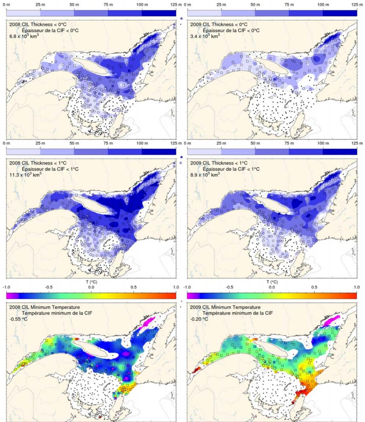
Fig. 24. Cold intermediate layer thickness ( $T < 0^\circ\text{C}$ , top panels;  $T < 1^\circ\text{C}$ , middle panels) and minimum temperature (bottom panels) in August and September 2008 (left) and 2009 (right).
