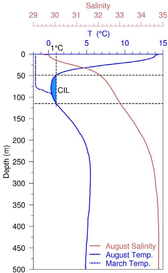
Fig. 2. Typical depth profile of temperature and salinity observed during the summer in the Gulf of St. Lawrence. Profiles are averages observed in August 2007 in the northern Gulf. The cold intermediate layer (CIL) is defined as the part of the water column that is colder than 1°C, although some authors use a different temperature threshold. The dashed line at left shows a winter temperature profile measured in March 2008, with near-freezing temperatures in the top 75 m.
