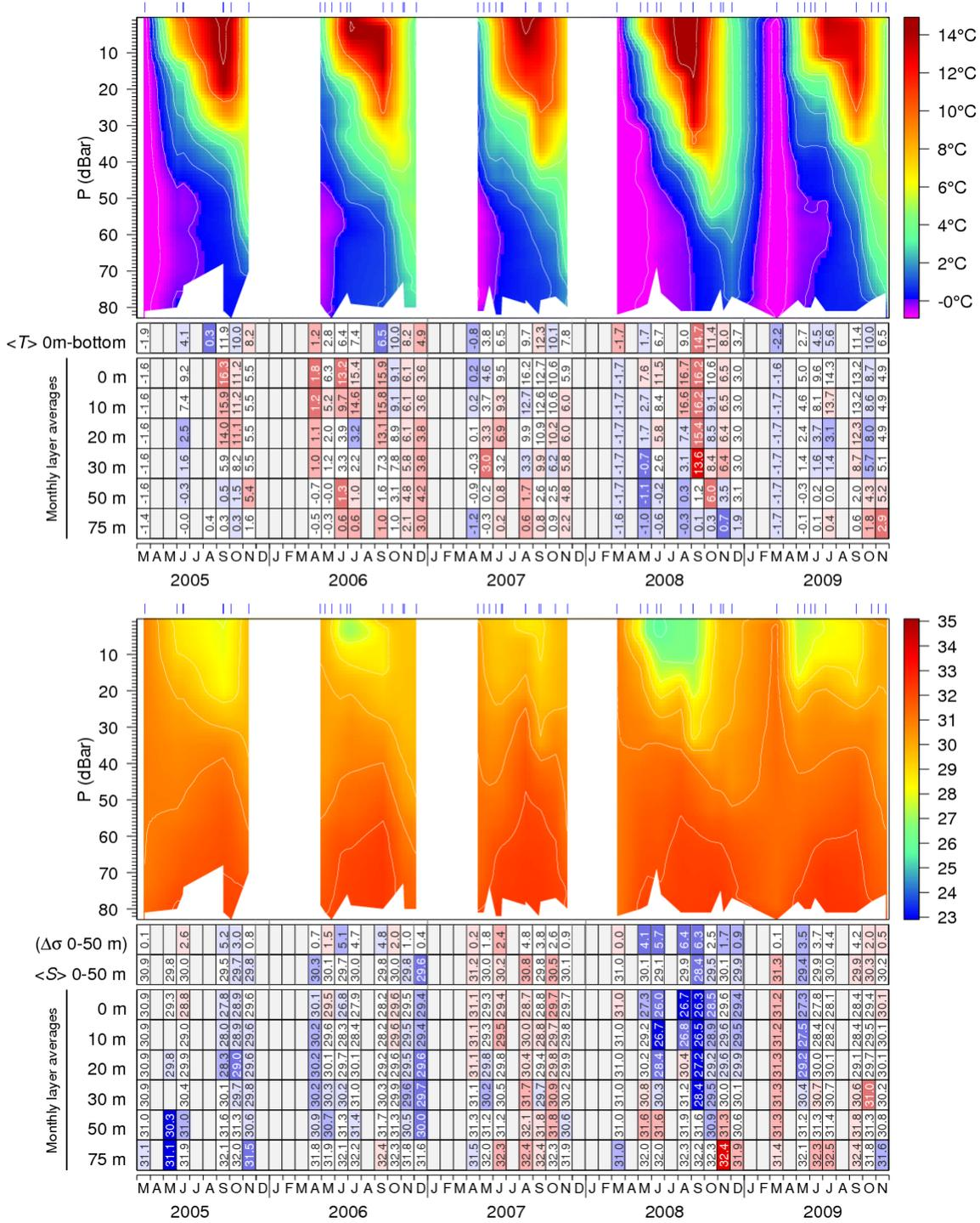
Fig. 45. Isotherm (top) and isohaline (bottom) time series at the Shediac Valley station; tick marks above indicate sample dates. Scorecard tables are monthly layer averages colour-coded according to the anomaly relative to the 1971-2009 monthly climatology for the station.
