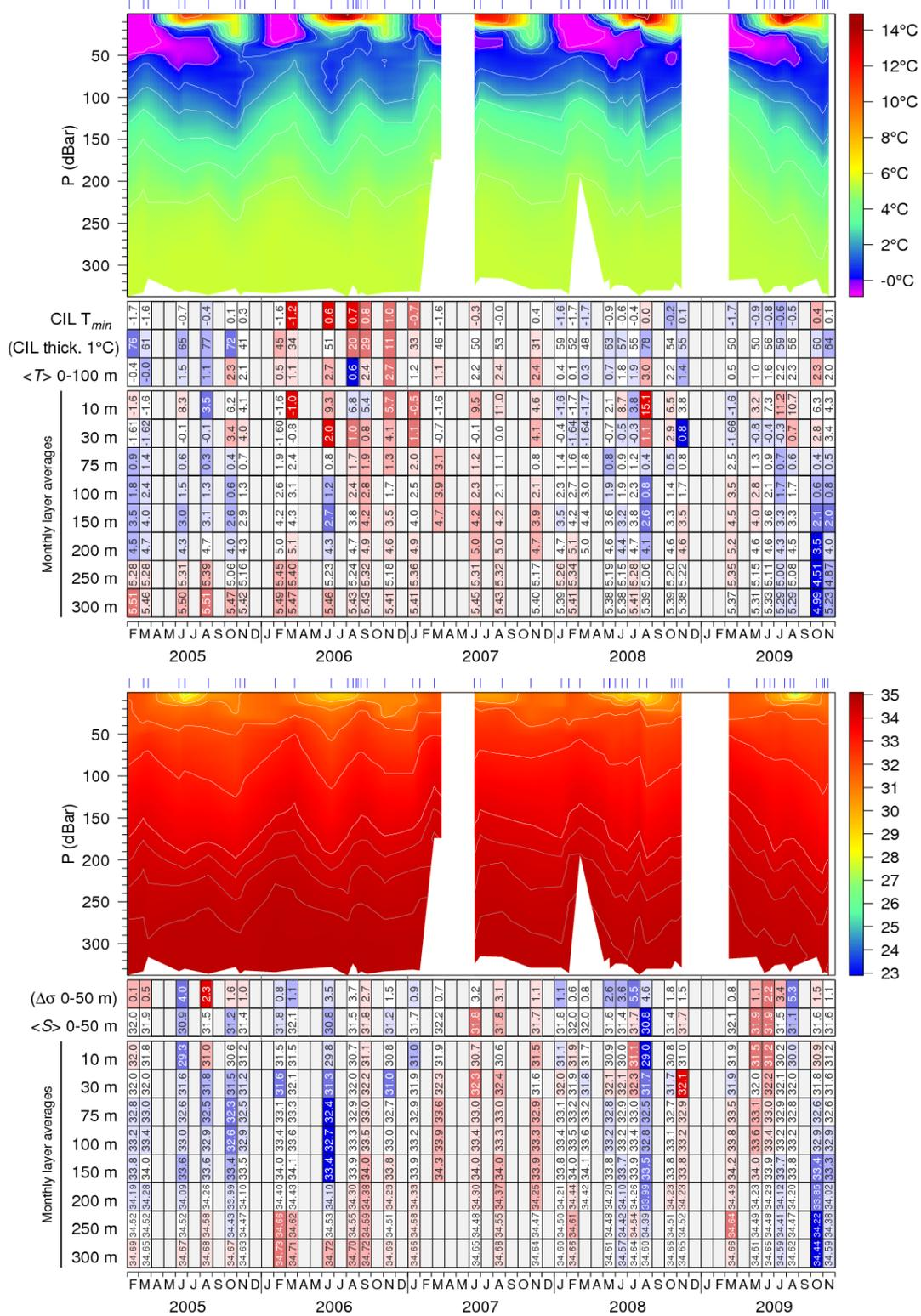
Fig. 44. Isotherm (top) and isohaline (bottom) time series at the Anticosti Gyre station; tick marks above indicate sample dates. Scorecard tables are monthly layer averages colour-coded according to the anomaly relative to the 1996-2009 monthly climatology for the station (yearly climatology for 250 m and deeper).
