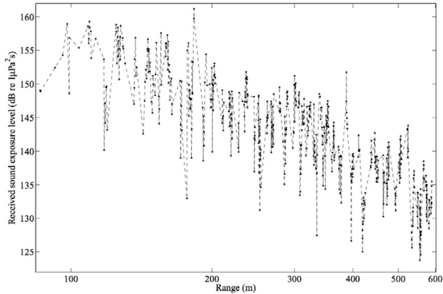
Figure 1. Received sound levels decline with distance from a Lofitech AHD source, although this decline is not consistent, and exhibits at least a 10-15 dB variation. Figure 5 in Shapiro et al. (2009).
