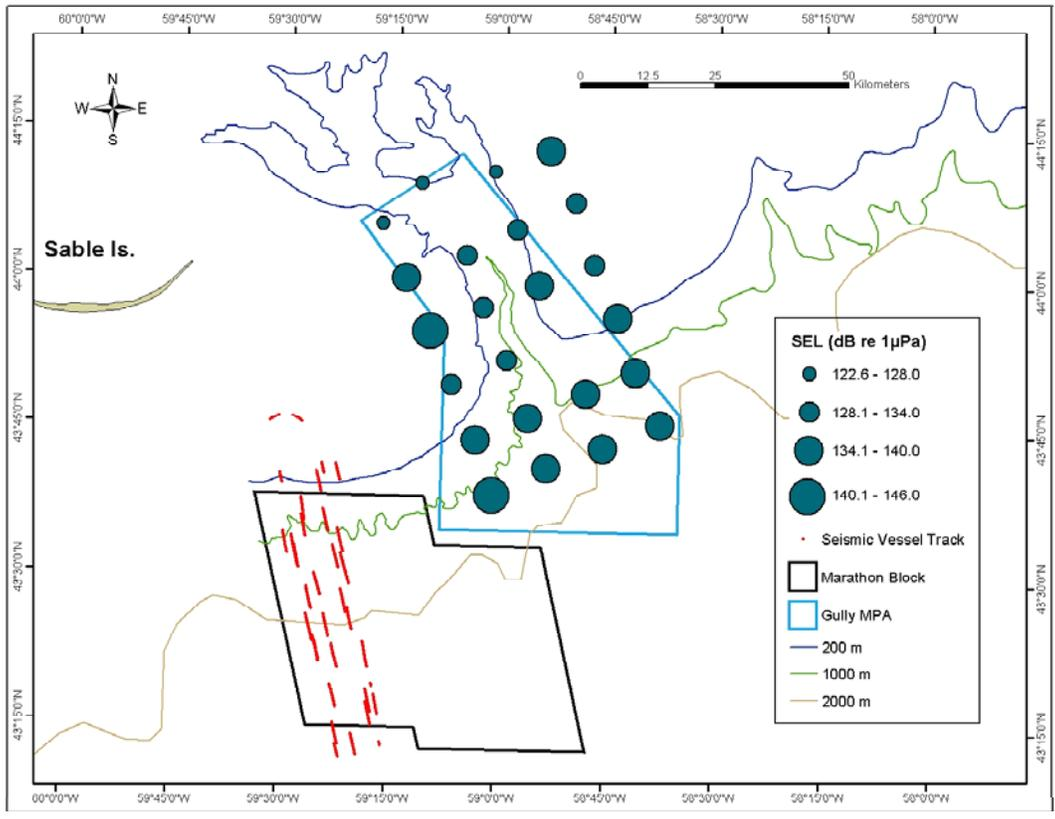
Figure 3. Geographical variation in measured average sound exposure levels (dB re 1  $\mu$ Pa) of seismic pulses (10-1000 Hz) emanating from within the Marathon Block in 2003. Data from COOGER Gully Project (McQuinn et al. 2004).
