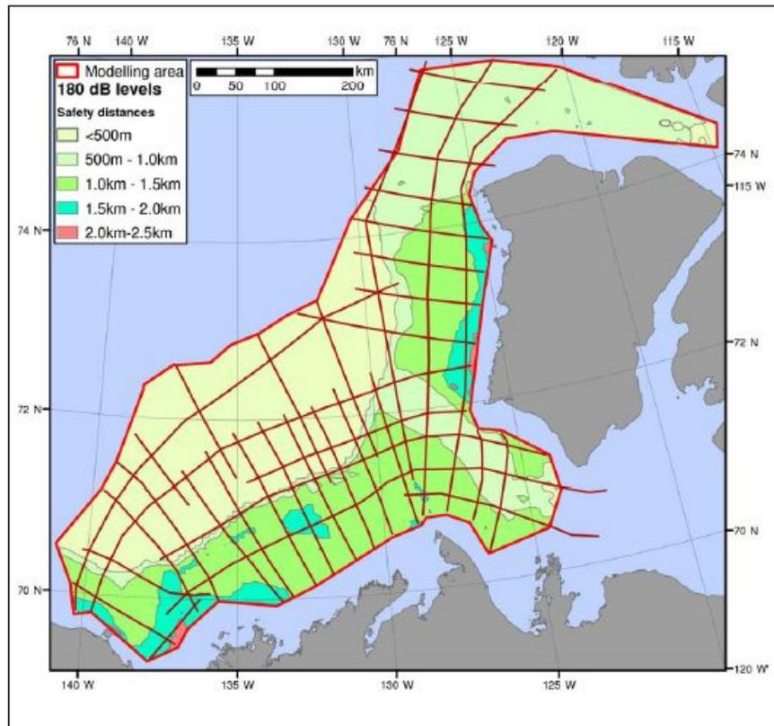
Figure 2. Modelled 180 dB re  $\mu\text{Pa}$  rms safety radii for the geophysical survey project to be conducted in 2009 as part of the Beaufort Span phase 2 survey (from LGL Limited, Env. Res. Assoc. 2008).
