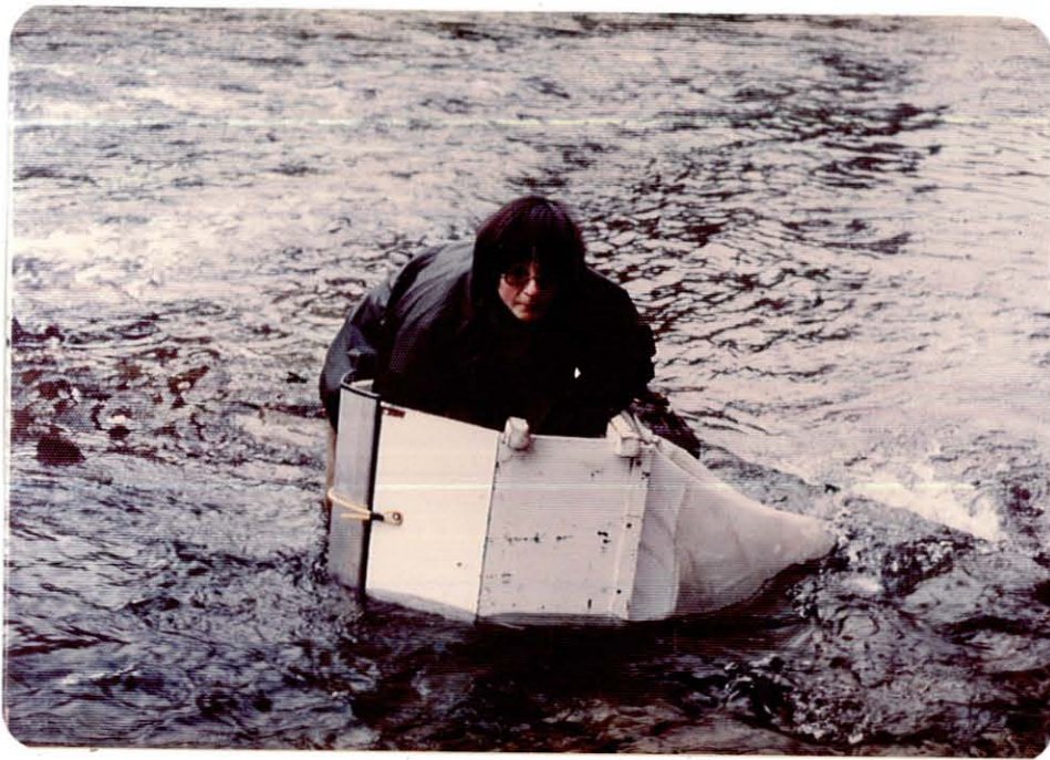
Plate 3. "Mundie" benthic invertebrate sampler in use in stream riffle.
