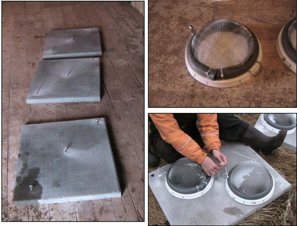
Figure 1. Field structures used in the experiment on herbivory effects on Chondrus crispus in Basin Head lagoon, 2007. Photos show concrete patio slabs with eye bolts (left image), stainless steel flour sifters turned into herbivore exclusion cages (upper right image), and attachments of paired cages containing Irish Moss on each patio slab (one coarse mesh, one fine mesh; bottom right image).
