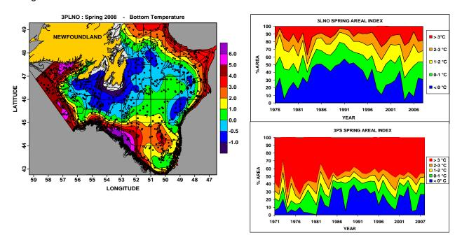
Fig. 8. Bottom temperature map ( $^{\circ}$ C) for the spring of 2008 for NAFO Divisions 3PLNO and the percentage area of the bottom covered by water in different temperature ranges.
