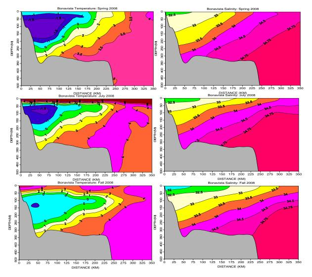
Fig. 6. Cross sectional contour maps of the temperature and salinity structure on the Eastern Newfoundland Shelf off Cape Bonavista during the spring, summer and fall of 2008.
