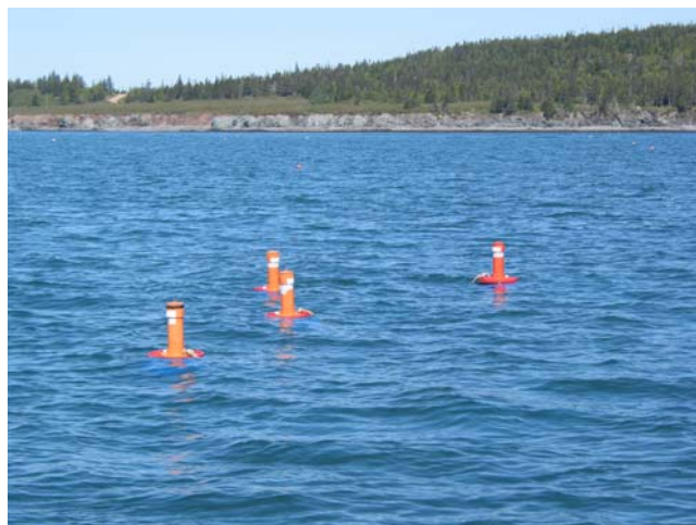
Fig. 2. Convertible Accurate Surface Tracker (CAST) drifters out of the water (left) and in the water (right). The central orange cylinder contains the electronics package including the GPS receiver and the ARGOS transmitter.
