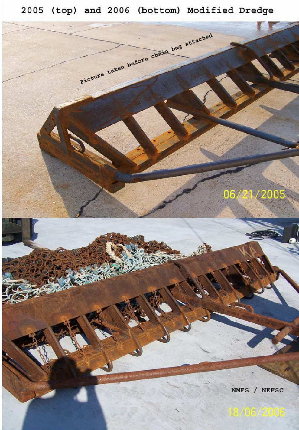
Figure 4. Turtle exclude scallop dredge frame design (with permission from R. Smolowitz).
