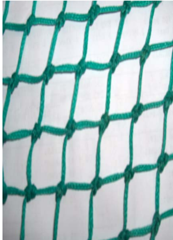
Figure 7. Difference in mesh opening for the same netting. Left photo is normal knotted diamond mesh and right photo is a knotted diamond mesh hung square, i.e., rotated 45 degrees. The netting is not under load.
