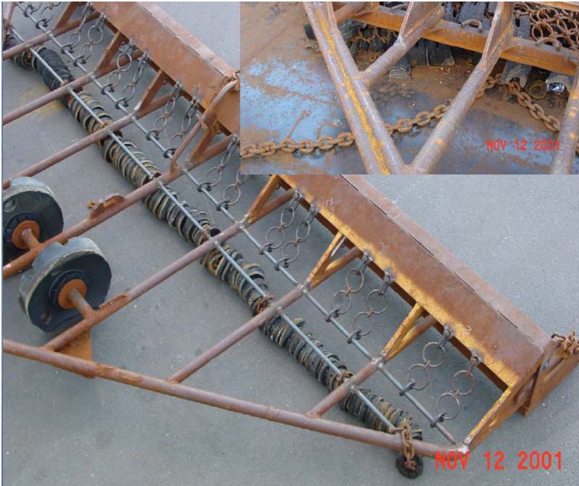
Figure 2. The 2001 dredge frame design showing cookie sweep and excluder rings (Smolowitz et al. 2001, used with permission from R. Smolowitz, Coonamessett Farm.
