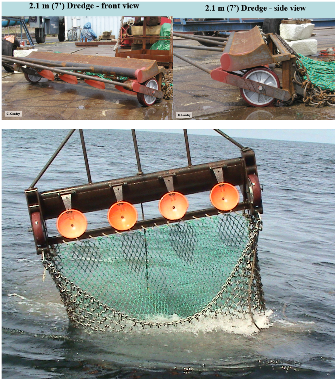
Figure 5. Seven foot hydrodredge developed at M.I.T. (Goudey et al 2006; used with permission).
