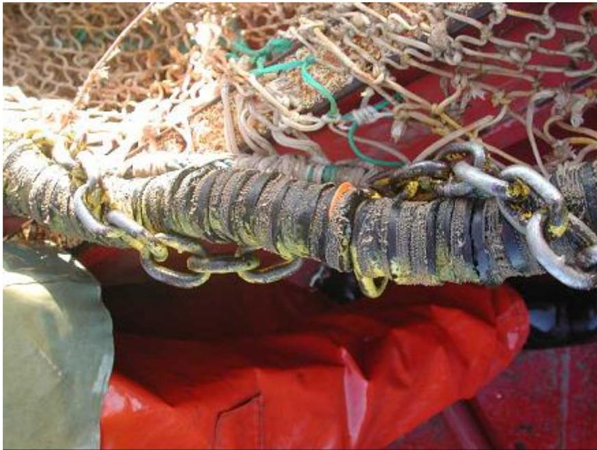
**Figure 10.** Trawl net showing the arrangement of chains rolled up to the foot rope since 1991.
