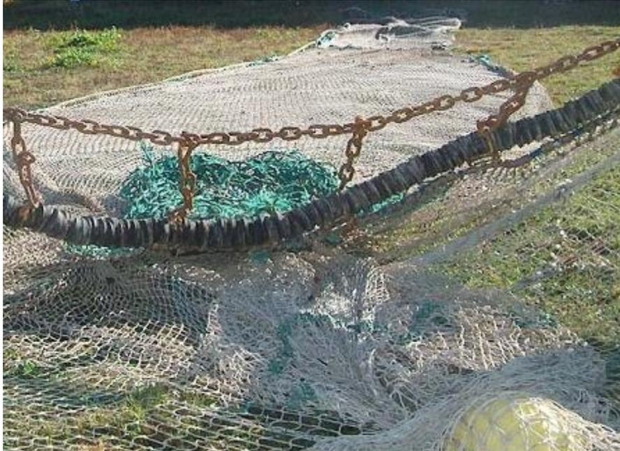
**Figure 9.** Trawl net showing the arrangement of chain attached to the foot rope from 1998 to 1990.
