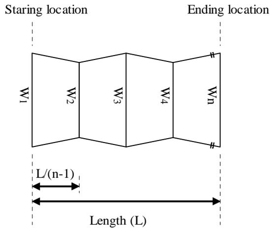
**Figure 14.** Swept area calculated using equally spaced trawl widths.
