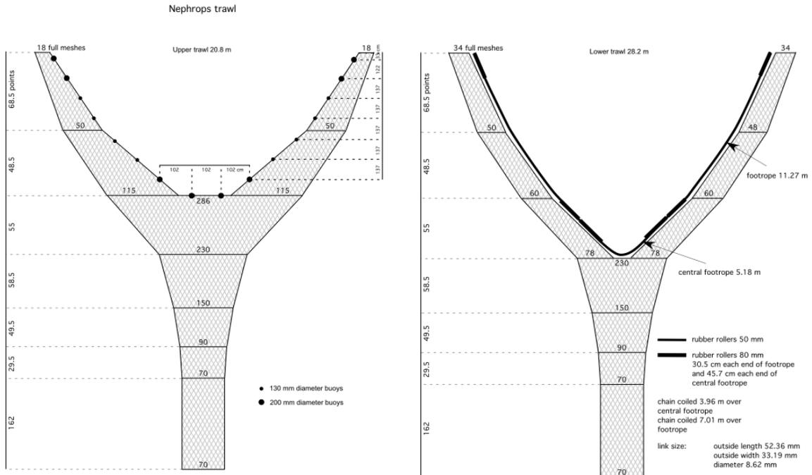
**Figure 8.** Nephrops trawl net diagram.
