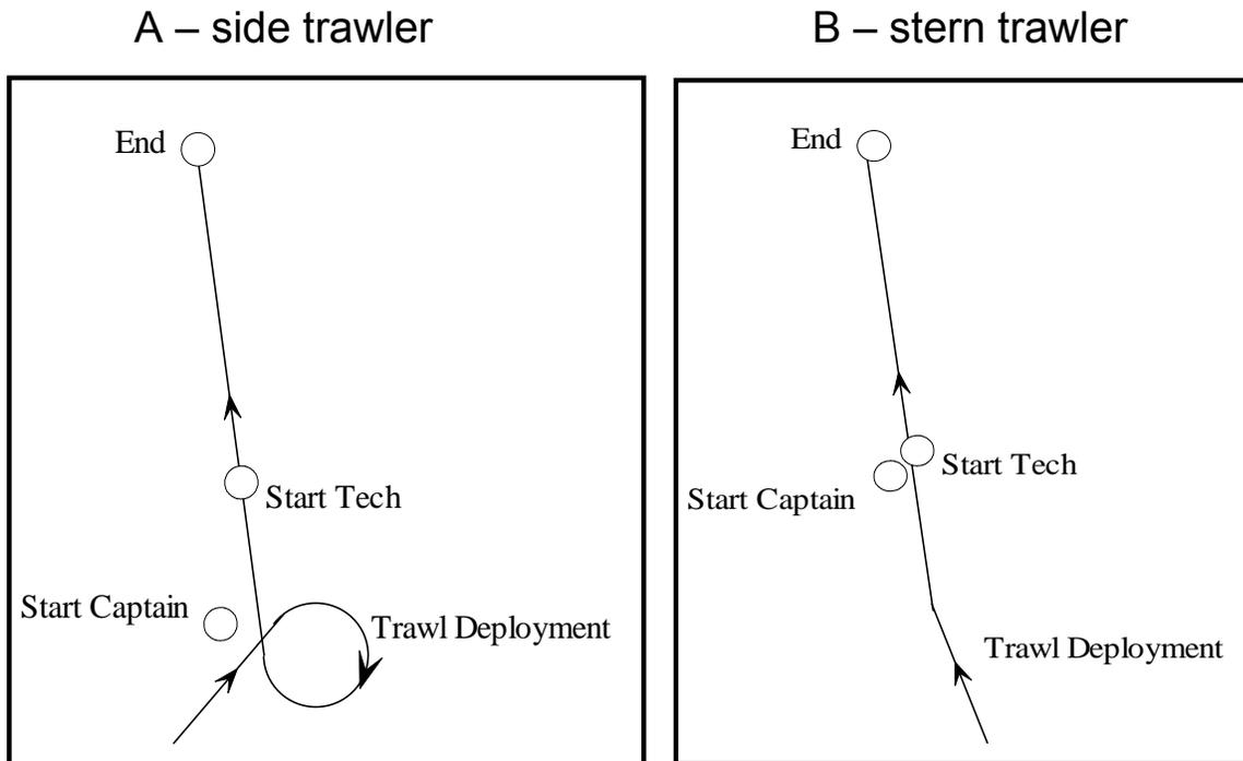
**Figure 11.** Diagram showing the different methodologies used in deploying the trawl net and determining the start and end time with : A, the side trawler (Emy-Serge) and B, the stern trawlers (Den C. Martin and Marco-Michel).
