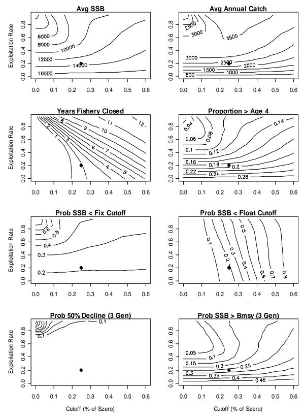
Figure 10. Queen Charlotte Islands contour plots showing results from the eight performance indicators for the Ricker S-R function with annually varying M and an extra year lag in fisheries after rebuilding above cutoff. Dots indicate the current harvest policy.
