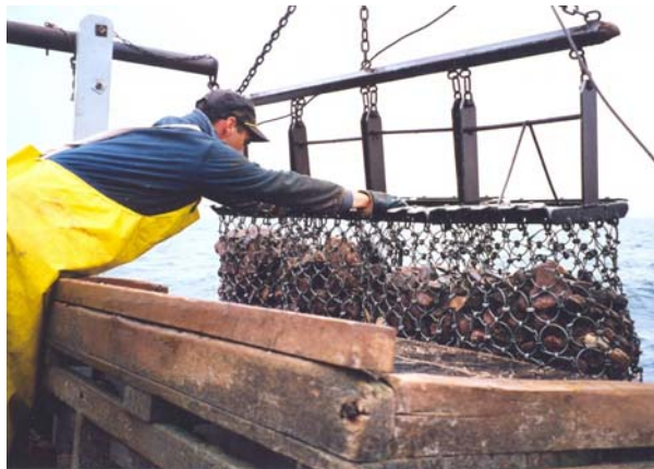
Figure 6. Digby-type drag most commonly used by fishers in the Gulf Region.
