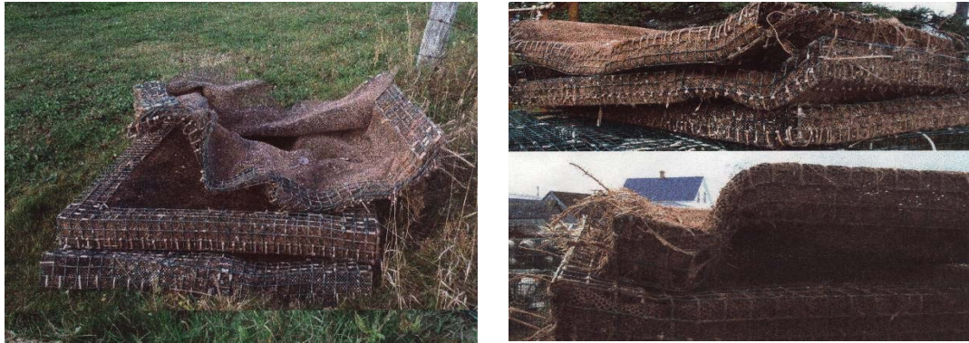
Figure 72. Badly bent trays occurring when cages tipped over.
