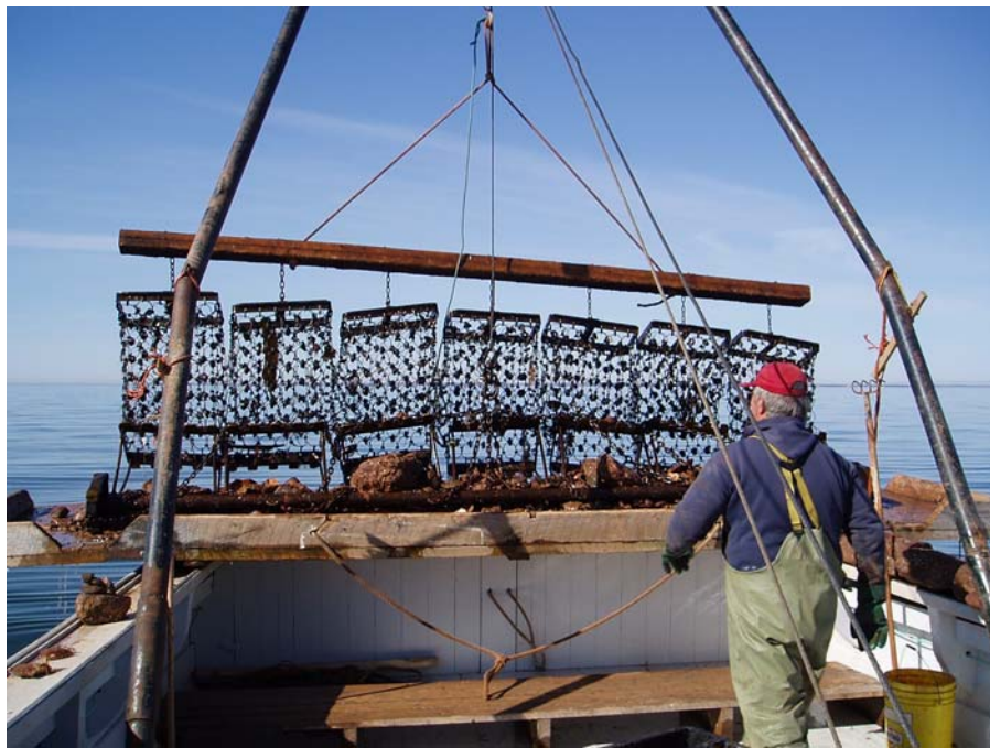
Figure 12. Seven bucket Digby-type scallop dredge used in the Gulf Region.
