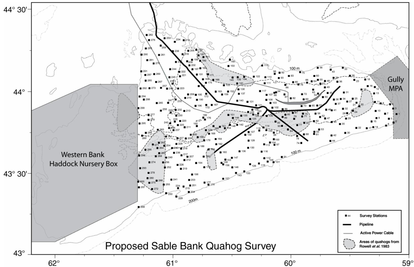
Figure 2. Station locations on Sable Bank showing areas of high quahog densities from Chaisson and Rowell (1985) and locations of other structures and areas that affect station locations for the 2003 ocean quahog survey.
