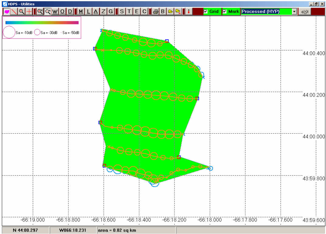
Figure 36. Acoustic survey transects and estimated total survey area of 0.82 km 2 for Trinity Ledge on Sept. 6, 2005 by the Sea Quiz .
