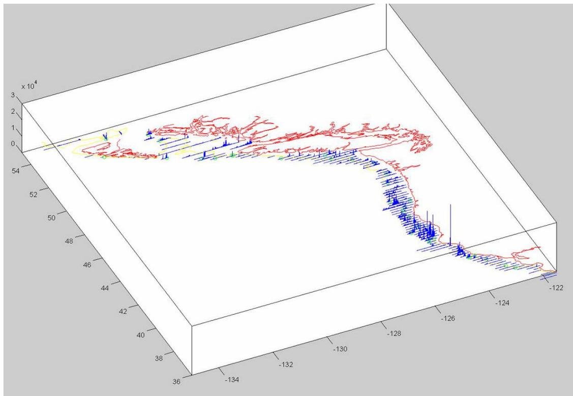
Figure 53. Plot of joint Canada-U.S. Pacific hake acoustic-trawl survey conducted by the US FRV *Miller Freeman*, June 15 – August 20, 2005. Horizontal blue lines show survey grid; vertical blue lines indicate distribution of hake along transects. Line height is scaled to maximum recorded acoustic backscatter level (SA;  $m^2/nmi^2$ ).
