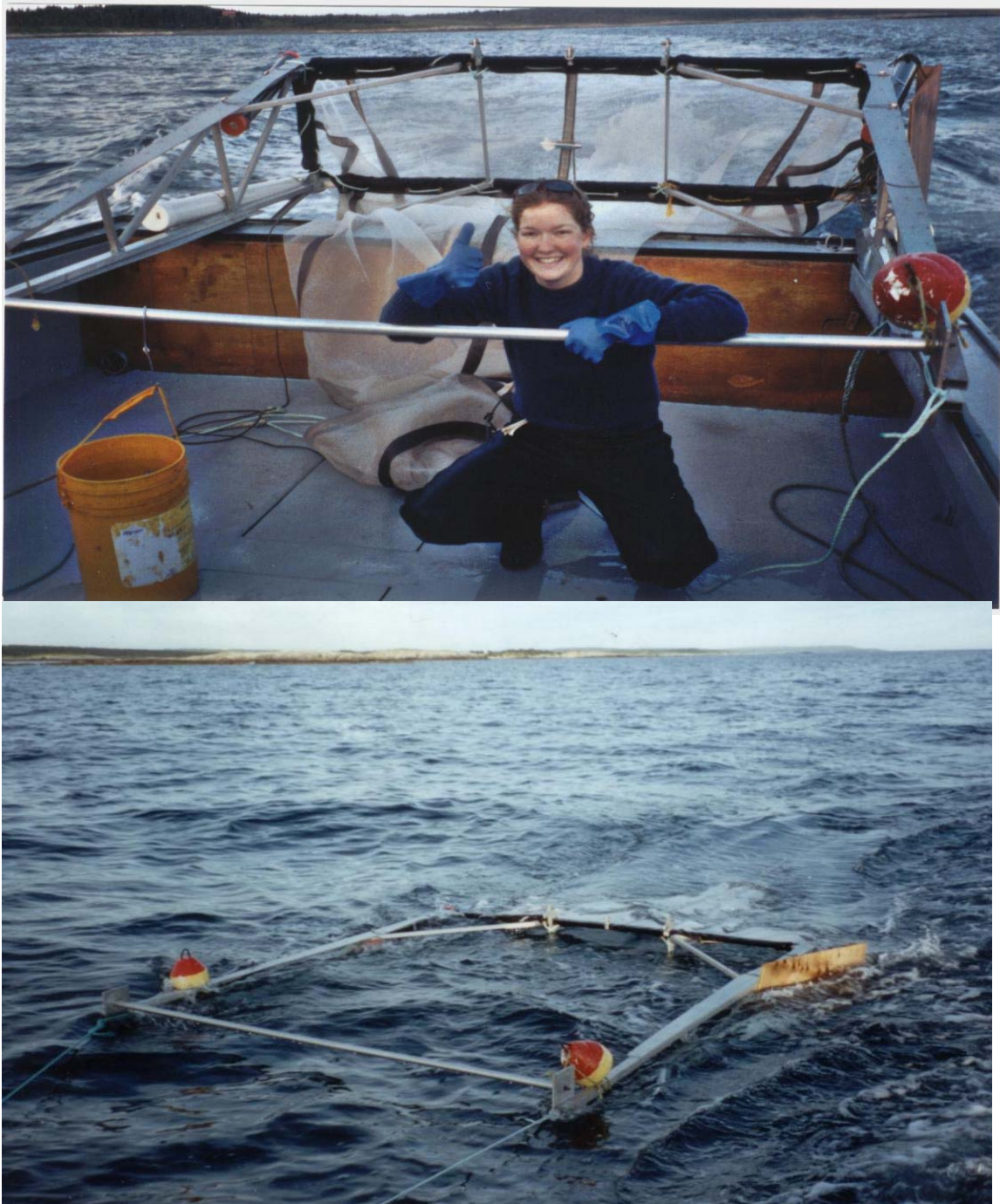
Fig. 4. Larval sampling net on the stern of lobster boat with intern (top); net fishing (bottom).
