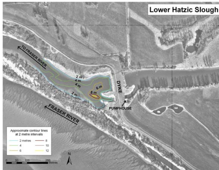
Figure 5a. Orthophoto (2001) of the mouth of Hatzic Slough, lower Fraser River, showing dike constructed for flood control. Reproduced with permission of D. Ham, Department of Geography, University of BC. Depth contours (m) from Lane and Rosenau (1997).
