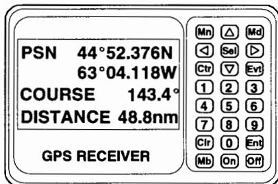
A constellation of 18 satellites reside in six circular orbits at an altitude of 20,000 km and a revolution period of 12 hours. At any location and time, there will be between 4 and 8 satellites over the horizon. Information from 3 satellites is sufficient to give a position, however a 4th satellite is required to give a position with certainty.
