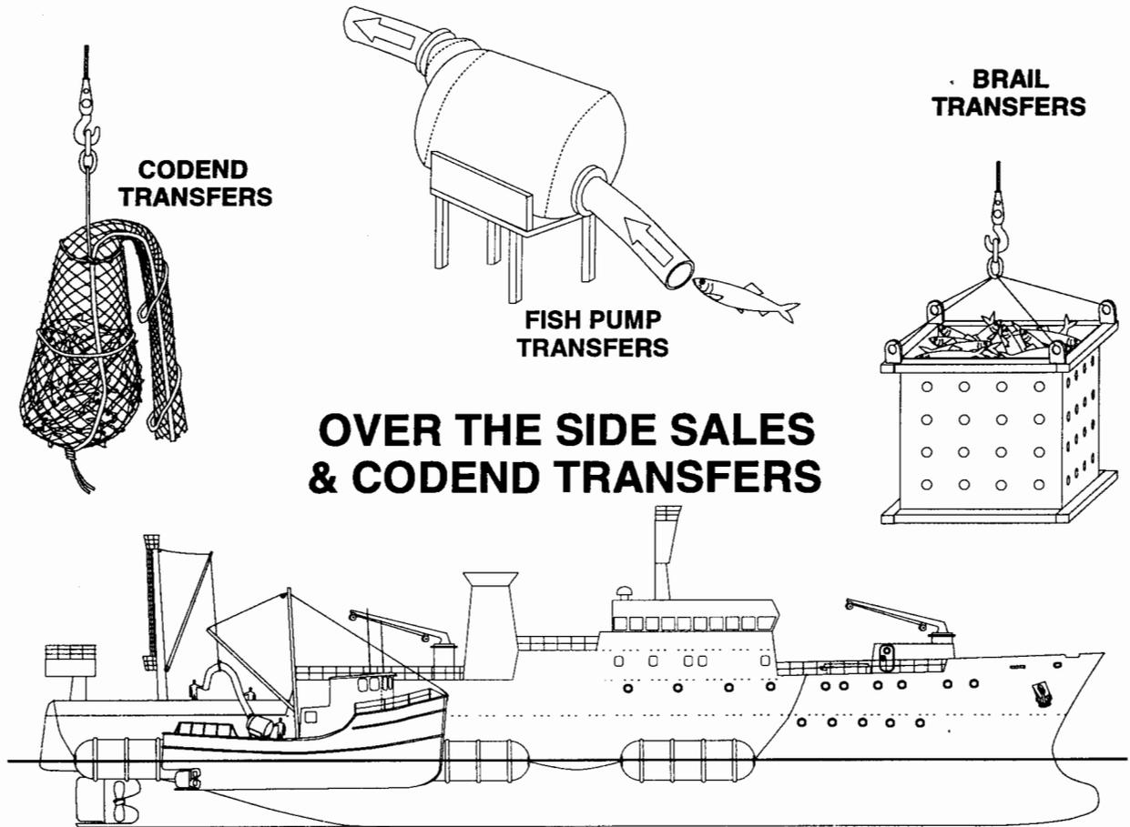
Codend transfers are used in joint venture fishing operations which involve a catcher and a processor vessel. The catcher, using a trawl net, conducts normal fishing operations to harvest the fish. When the tow has been completed the trawl is hauled back and preparations are made to transfer the codend.
