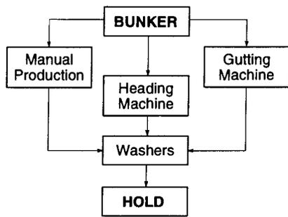
the vessel size and the directed fishery. For most domestic groundfish fisheries the processing is done by hand. The fish are dressed by cutting the belly flaps and cleaning out the entrails (referred to as gutting). The fish are then washed and "iced" in the hold. The larger offshore groundfish vessels may have one or more gutting and heading machines which dress (rip+gut) the fish automatically; it may only require one crew member to operate.
