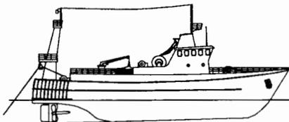
Offshore trawlers use bottom, off-bottom and midwater otter trawls to direct for groundfish, squid and small pelagic fish. Fishing activity can be determined by the presence of two cables (warps) extending from the stern of the vessel into the water. Fish processing on large offshore trawlers is done either by hand or with a limited amount of processing equipment such as gutting and deheading machines. Product types on these vessels is usually limited to round, gutted head-
