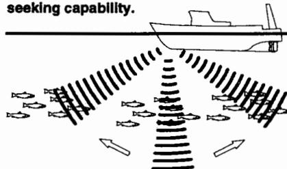
Sonar operates on the same principles as an echo sounder, except that signal direction from the vessel can be rotated horizontally 360°. Distance and bearings of underwater objects up to 2 miles from the vessel can be obtained as the sonar transducer is rotated. The signal can be angled downwards to track underwater objects approaching the vessel.
