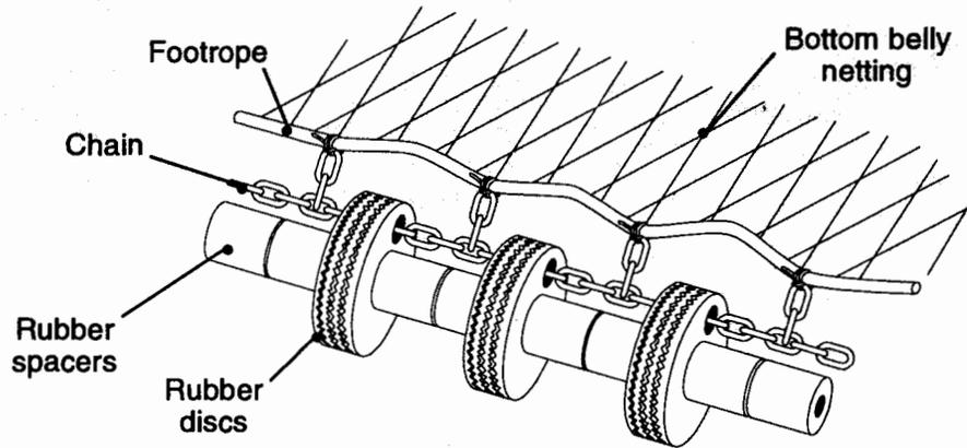
footrope. They are used exclusively on bottom trawls to prevent damage to the trawl by lifting the footrope and netting off the bottom and for rolling over obstacles.
