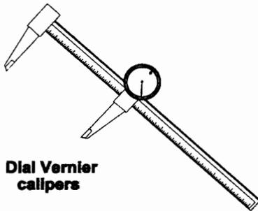
Calipers are required for length groupings measured in millimeters or  $\frac{1}{2}$  millimeters (shrimp, crab, clam or scallop). Calipers allow for very exact measurements. Three types of calipers used by Observers are:
