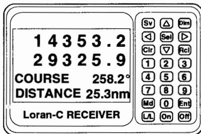
Loran C (long range navigation) is a radio navigation system that operates from low-frequency pulses over a long range.
