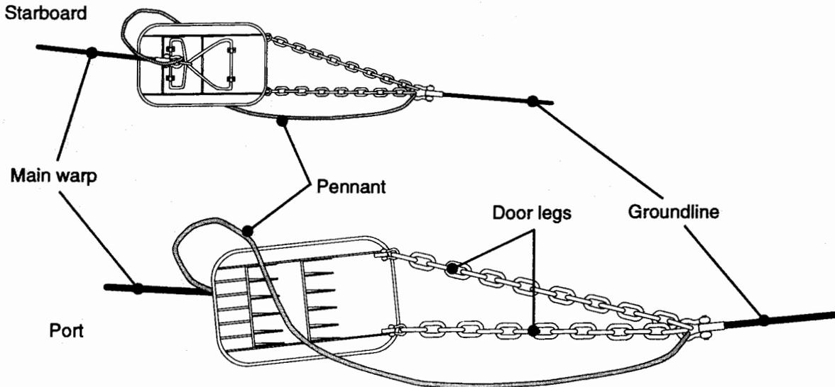
The *pennant* is a cable loosely attached at the point where the door legs meet the groundline, and to the inside of the doors. The purpose of the pennant is to facilitate the deployment and retrieval of the trawl.
