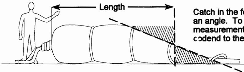
Catch in the forward part of codend settles on an angle. To compensate for this the length measurement is taken from the end of the codend to the mid point of the forward angle.
