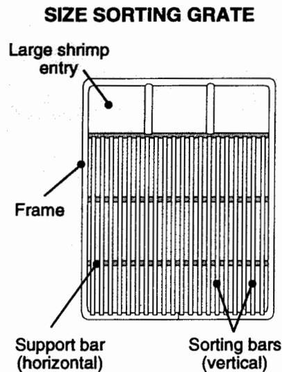
In recent years a separator grate capable of sorting by size has been introduced to the shrimp fishery. This arrangement includes a second grate in the lengthening piece inserted directly behind the bycatch reduction system. The size sorting system is similar to the bycatch grate with a few variations. This system includes a size sorting grate, two panels of netting and an escape exit.
