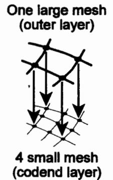
codend mesh. Each flap of netting must be no more than 10 mesh long and at least the width of the codend. The net flaps are attached across the top of the codend by the leading edge with the opposite end trailing over the flap directly behind it.
