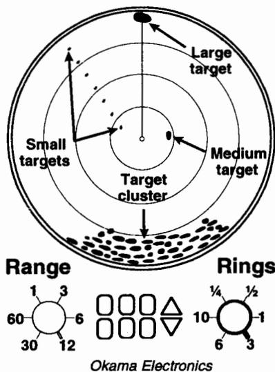
The word RADAR is an acronym of Radio Detection and Ranging. The basic principle of radar is the property of reflectivity of objects to radio waves. Radar enables reflective objects to be revealed and the position becomes known. From this position, radar can provide information on distance and direction of the target being displayed.
