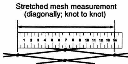
Gillnets are selective in terms of mesh size; the larger the mesh the larger the size of fish retained. Mesh size is measured from the inside corner of one mesh to the diagonally opposite corner. Although not specified in the regulations, it is recommended that at least 20 meshes be measured to give a fair representation of the net mesh size.
