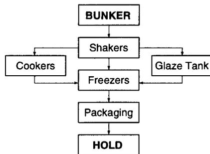
Fisheries such as offshore shrimp and clams have a complex processing operation. Once the shrimp are brought on board they are dumped in a holding tank filled with water. From the tank the shrimp pass through shakers that sort the catch by size. Shrimp are processed in to three product forms, depending on size; premium (large), cooked (medium), and industrial (small). The size is determined by number of shrimp per kilogram.
