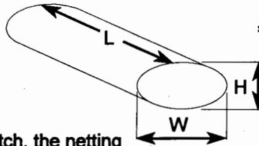
Codend shapes vary with amount of catch, the netting materials used and size of the net. Use the volumetric shape that most closely resembles the filled portion of the codend.
