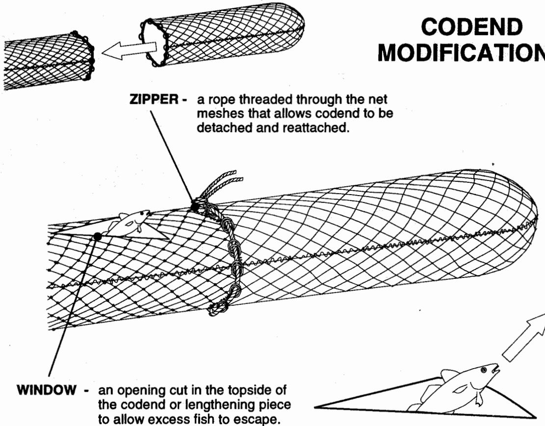
the codend fills as far as the window the strain of the catch breaks the twine, opening the window. Any fish caught subsequent to this simply exit unharmed through the window. The further the distance of the window from the codline, the more fish will be retained in the net.
