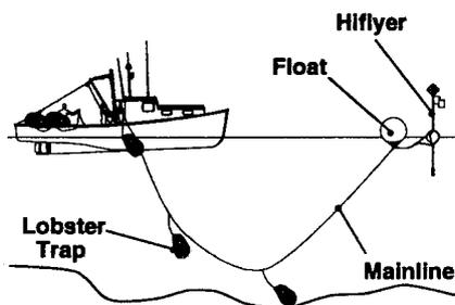
Lobster traps, also referred to as *lobster pots*, vary in design and size from region to region. Older styles used mainly for inshore fishing consist of a frame constructed from pieces of wood (laths) and cotton or nylon twine. Each trap is equipped with one or two openings allowing the lobster to enter but situated so escape is prevented. The common design of traps used today consist of a rectangular metal frame covered with wire mesh. Entrances are located on each side of the trap.
