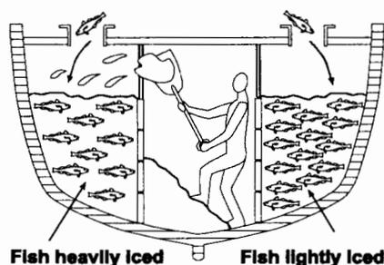
The procedure used to perform a hold check will depend on the vessel type. The majority of domestic wet fish trawlers store the catch in pens. Determining the capacity of these pens will provide the Observer with an estimate of kept weight. The Observer can determine the pen capacity by:
