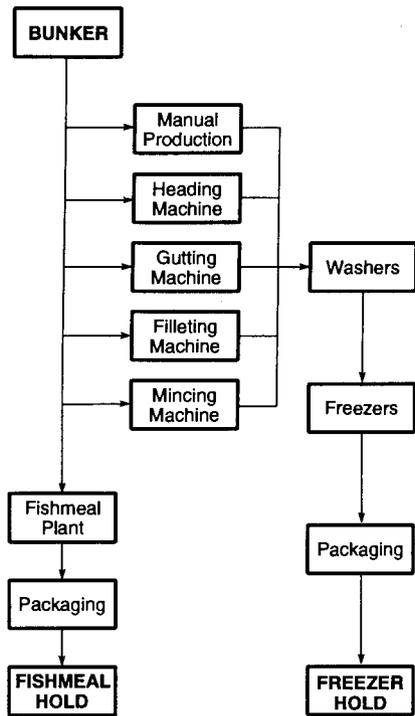
fed into this chute along with unmarketable bycatch and damaged fish. Once the bunker is full to a sufficient level, the contents are passed through the meal plant machinery. The offal is pressed until the moisture is removed and dried. The end result is a powdered product which is packed in bags and stored in the holding area. Bags of fishmeal generally weigh 30 to 50 kilograms.
