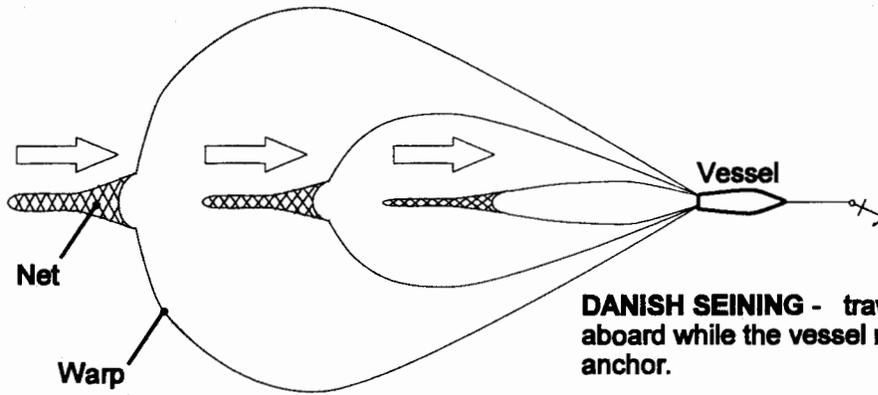
**DANISH SEINING** - trawl seine net is winched aboard while the vessel remains stationary at anchor.
