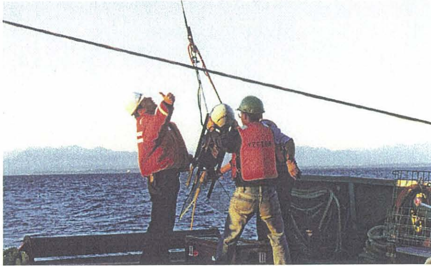
Figure 2.4: 330 kHz steerable sidescan towfish during deployment from the stern of the CCGS Vector.
