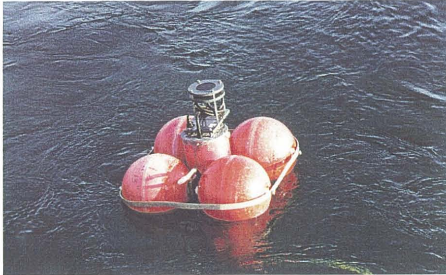
Figure 2.5: Self-contained WASP instrument with 4 floatation spheres. The 200 kHz transducer is the black disk within the topmost support bracket.
