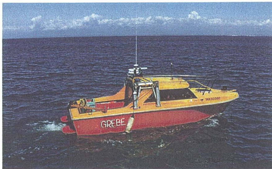
Figure 2.3: Survey launch Grebe used for supplemental EK-500 echo-sounder surveys. The 120 kHz transducer was mounted on a para-vane (not visible in photo) beneath the starboard side support frame.
