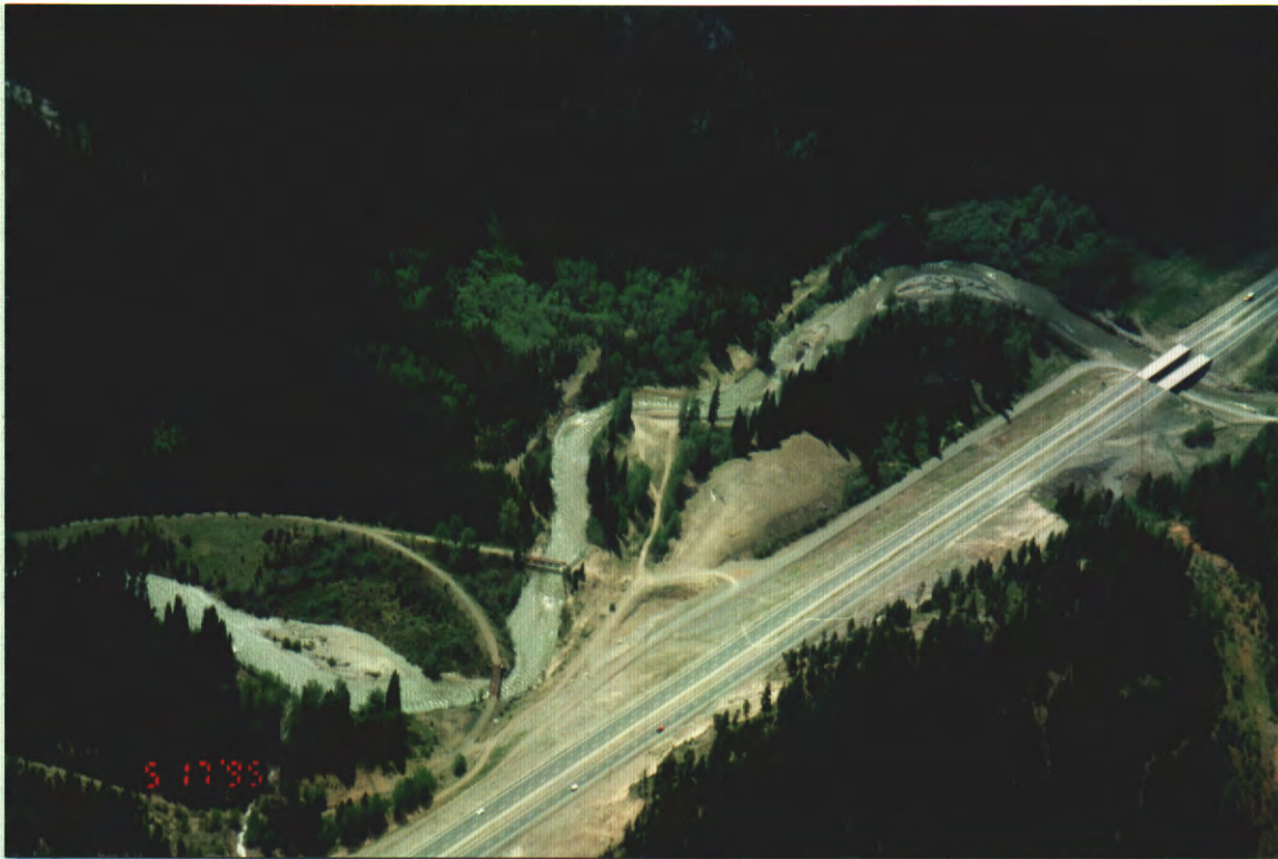
PHOTO 6. Linear corridor consisting of the Coquihalla Highway, abandoned railway, 2 oil/gas pipelines and the B.C. Tel fibre optic line have constrained the Coldwater River (Photo by M. Crowe).
