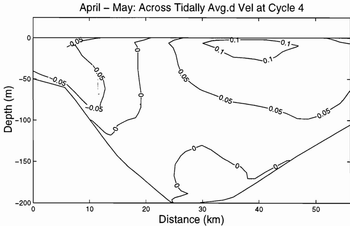
**Fig. 6.1.5b. Prognostic calculation of the density and current distributions across the Gully averaged over the fourth M2 tidal cycle. Positive velocities are directed into the page.**
