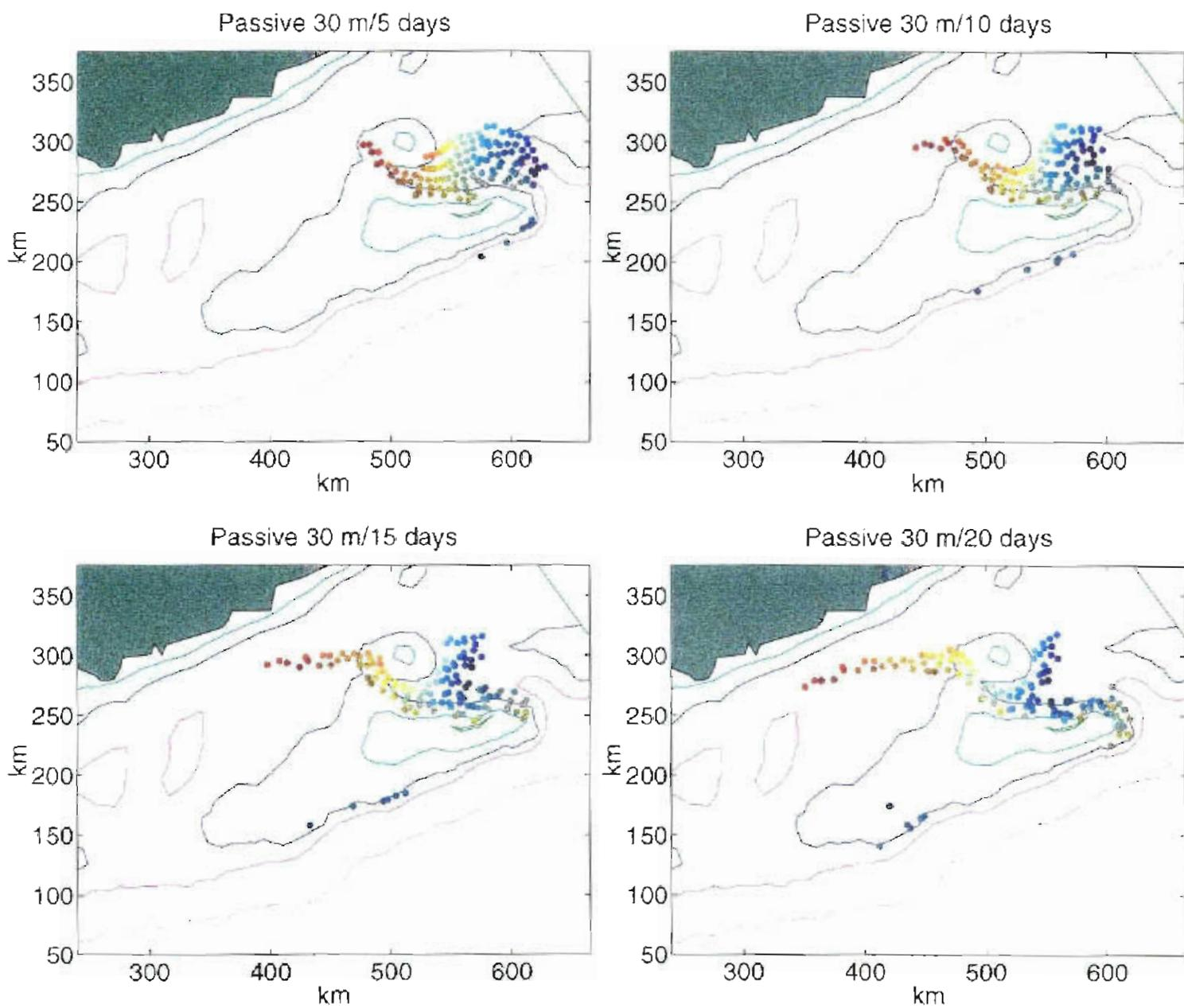
Fig. 6.1.6d. Particle positions every 5 days for days 5 to 20 when allowed to adjust to vertical velocities. Initial depth of particles was 30 m.
