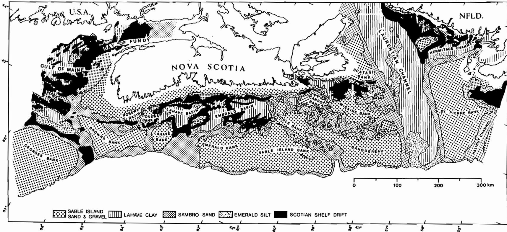
Fig. 3.0.2. The distribution of surficial sediments on the Scotian Shelf (King and Fader, 1986).
