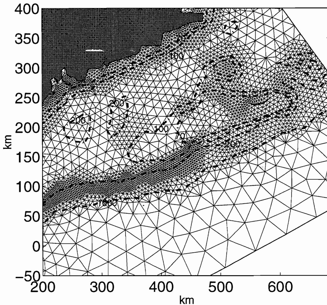
Fig. 6.1.2. Finite element model grid for the Eastern Scotian Shelf. The 100, 200 and 1000 m depth contours are shown.
