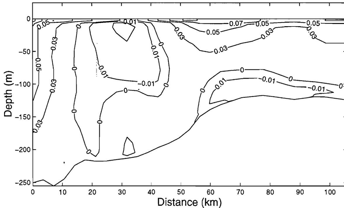
Fig. 6.1.5c. Prognostic calculation of the density and current distributions along the Gully averaged over the fourth  $M_2$  tidal cycle. Positive velocities are directed into the page.
