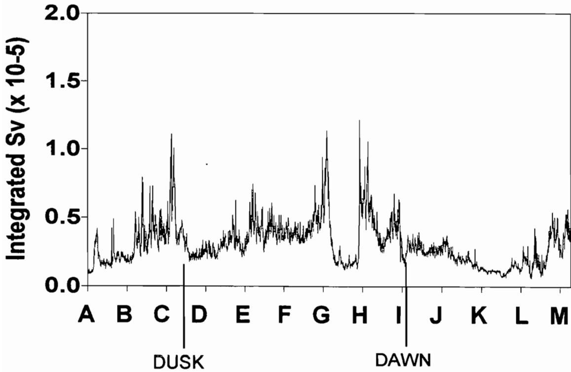
Fig. 6.3.20. Acoustic backscattering by macrozooplankton (>2.5 cm) from off Sable Island into the Gully in April 1997.
