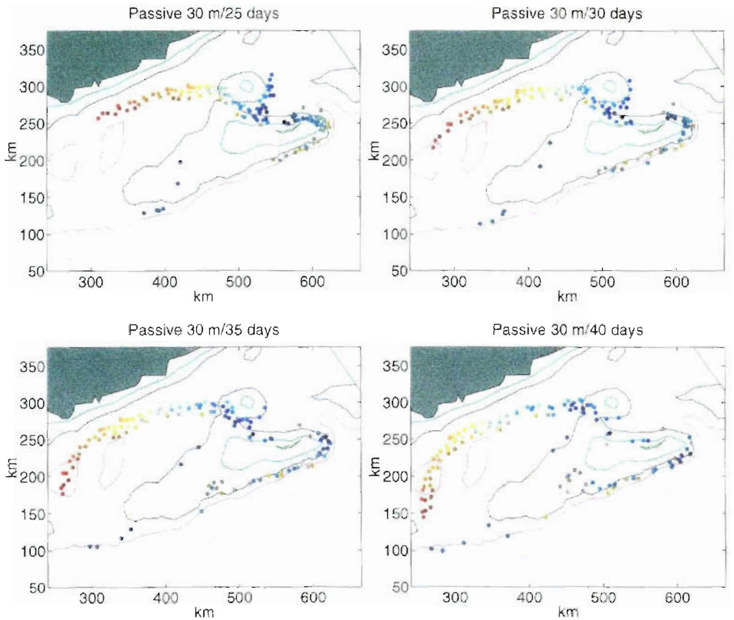
Fig.6.1.6e. Particle positions every 5 days for days 25 to 40 when allowed to adjust to vertical velocities. Initial depth of particles was 30 m.
