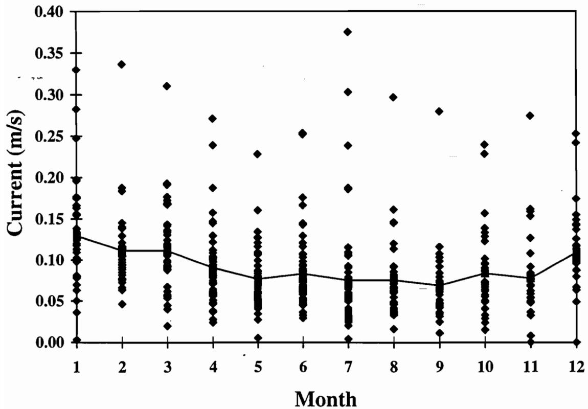
Fig. 6.1.9. Standard deviations of the low-frequency currents for the region shown in Fig. 6.1.1. The line indicates the mean value of the standard deviations.
