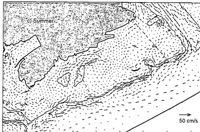
Fig. 6.1.3. Near-surface (averages between 5 and 25 m of the surface) mean currents for (a) winter, (b) spring, and (c) summer from model simulations with full forcing (From Han et al. 1996).
