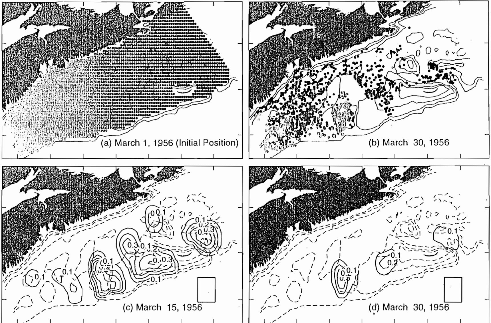
Fig. 6.1.8. (a) Initial positions of particles shaded with different intensities in gray to indicate starting positions; (b) Positions of particles after 30 days; (c) Retention index showing the proportion of particles remaining in a box of a given size (see bottom right corner) after 15 days; (d) Same as (c) but after 30 days. From Cong et al. (1996).
