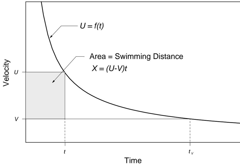
**Figure 6.2** Swimming distance based on  $X = (U - V)t$ .
