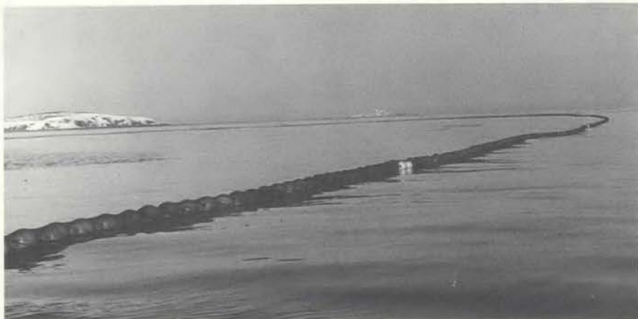
Seine net for containing oil slicks devised by the Industrial Development Branch of the Department of Fisheries and Forestry.
