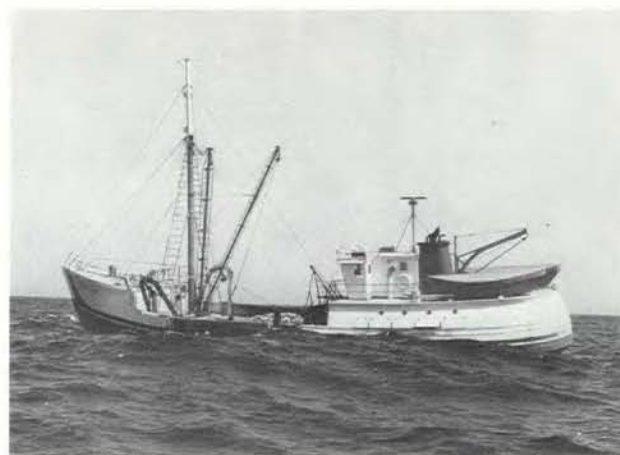
Fig. 4. - MV Stuart and Lynne, a 95-foot modern offshore scallop boat dragging Georges Bank.
