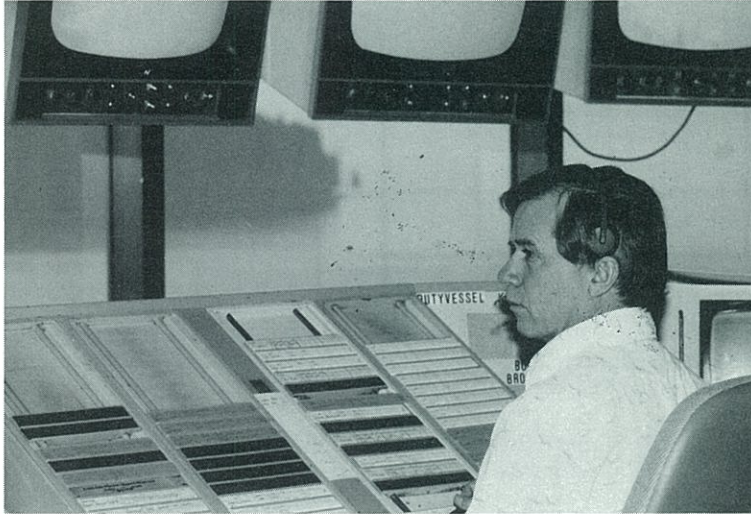
A Coast Guard MCTS officer, with transit-strip cards visible on his console, sits monitoring and controlling vessel traffic at the Vancouver Harbour console.
