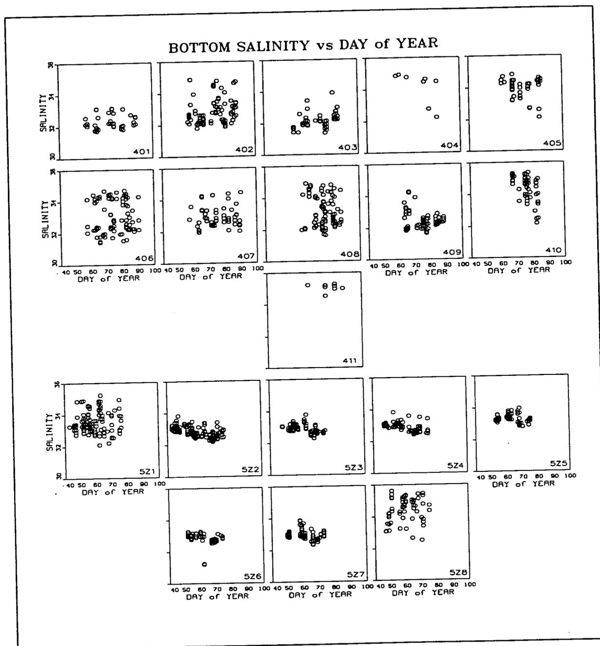
**Figure 8:** Near-bottom salinities within the spring 4VSW and 5Z surveys in relation to day of the year. The numbers and letters in the lower right hand corner of each panel indicate the survey stratum. Each open circle represents the values at one hydrographic station.
