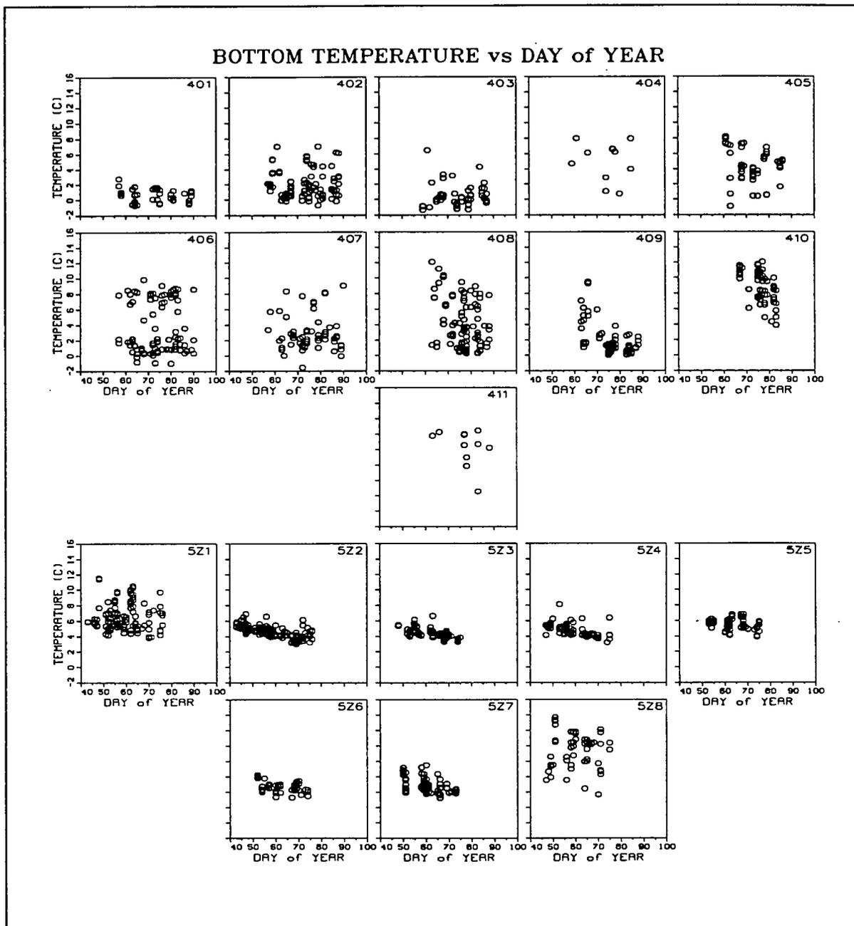
**Figure 7:** Near-bottom temperatures within the spring 4VSW and 5Z surveys in relation to day of the year. The numbers and letters in the top right hand corner of each panel indicate the survey stratum. Each open circle represents the values at one hydrographic station.
