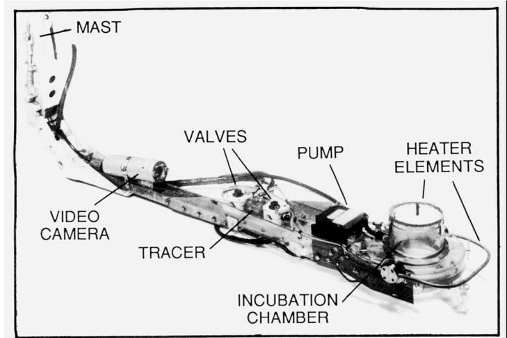
Fig. 5 The underice incubator used for measuring in situ growth rates of the underice algal layers.
