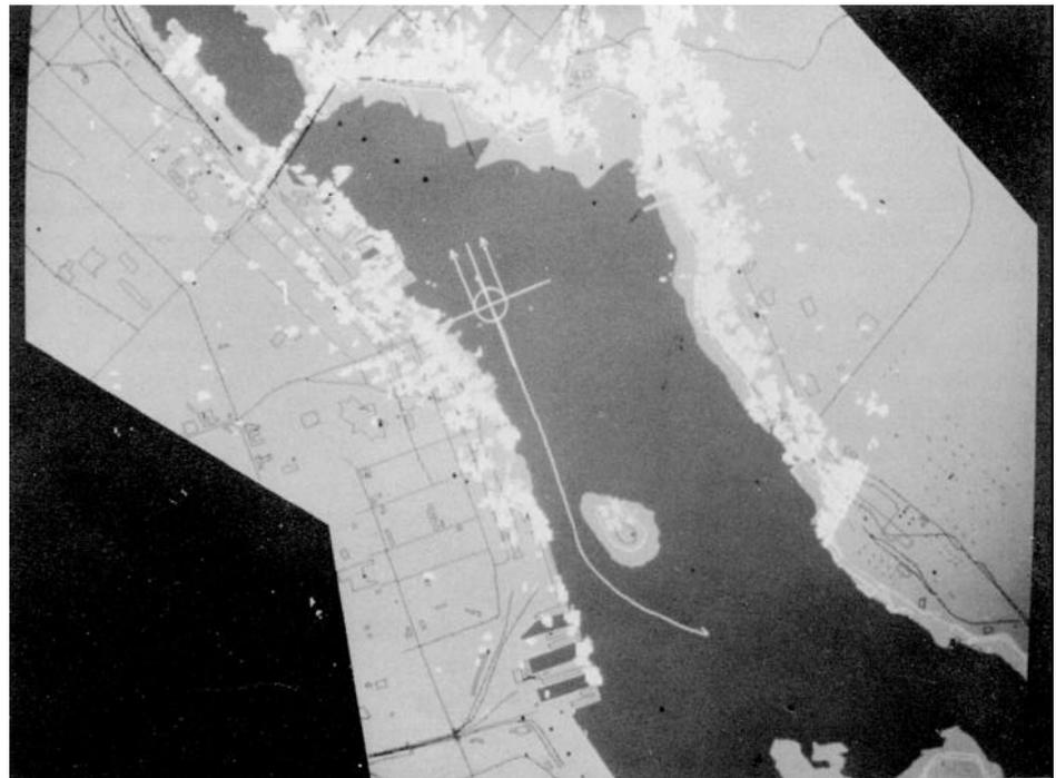
Fig. 1. Electronic Chart Testbed display of Halifax Harbour with radar. Ships symbol carries parallel index bars used to plot clear passage ahead. The radar is offset 30 m east from chart because ship is positioned by GPS NAVSTAR on new satellite datum whereas chart data was on old North American datum at that time.
