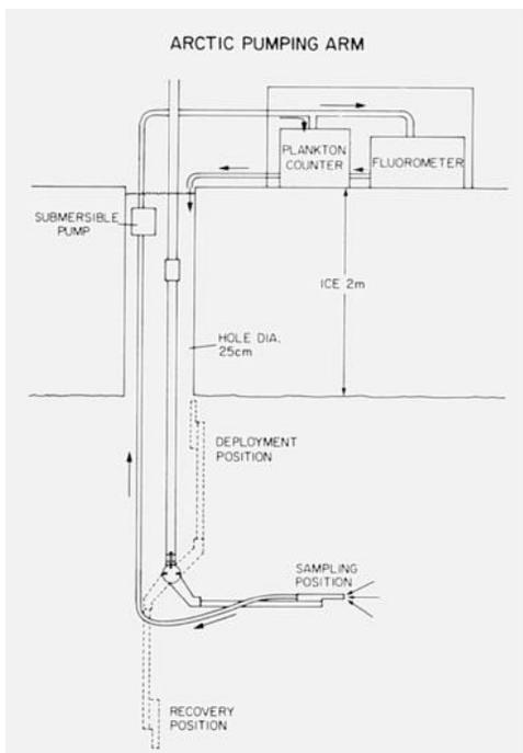
Fig. 2 The underice pumping arm used for sampling zooplankton. The operational zooplankton and chlorophyll were accomplished with a plankton counter and fluorometer on the ice surface.
