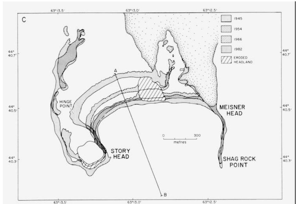
*Fig. 1 This beach at Storey Head, on Nova Scotia's Atlantic coast, is being monitored by coastal geologists based at the Atlantic Geoscience Centre. It has been moving landwards at an average rate of about 8 metres per year. Here the rise of sea level due to global change would add to the existing regional subsidence of 30 cm per century. Beaches such as this may be destroyed From Forbes et al (in review).*
