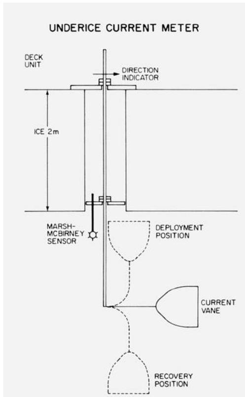
Fig. 9 An underice current meter capable of being deployed through a 24 cm diameter ice hole.
