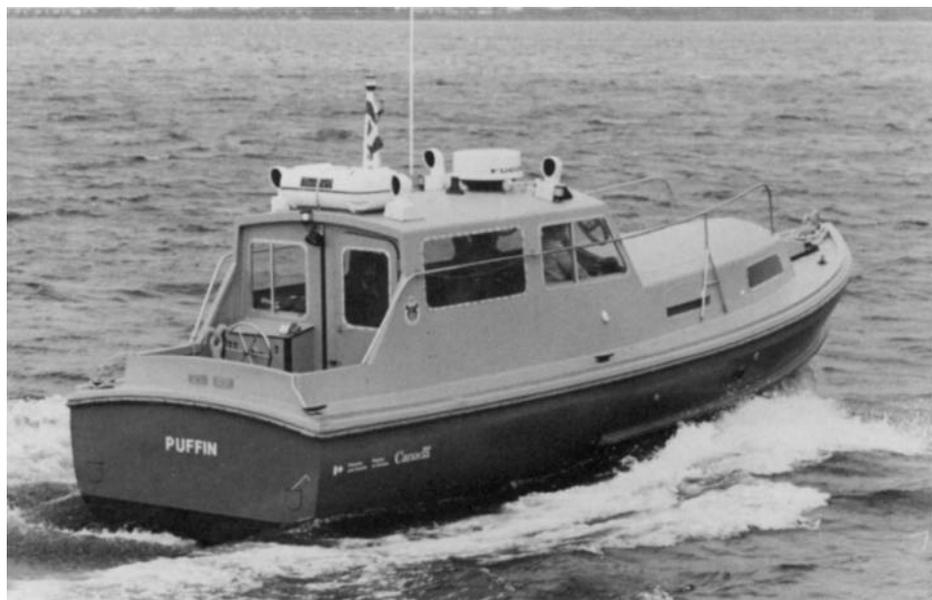
*C.S.L. Puffin is a new hydrographic survey launch; constructed of fibreglass, the semi-displacement, round bilge hull is capable of 20 knots full speed*
