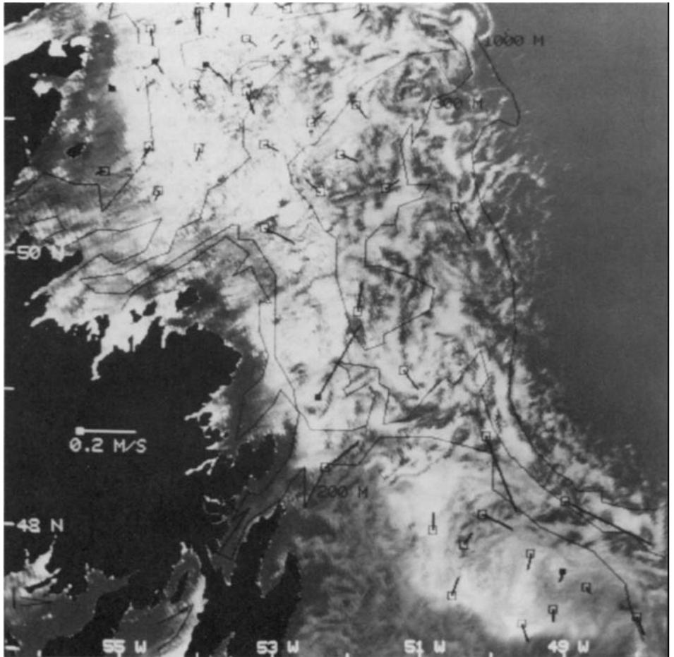
Computer monitor display of sea ice extent and movement off Newfoundland. Ice cover (white) is determined from a satellite image. Ice movement is estimated by comparing the positions of ice-field features during successive satellite overpasses (open arrows), and by monitoring positions of satellite-reporting beacons that were placed on the ice by helicopter (closed arrows).
