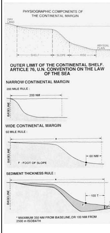
the shore to a point where the bottom abruptly begins to steepen. Worldwide, here is considerable variability, but the greatest average depth of the shelf is usually of the order of 200 metres, with a gradient of 1 in 1000.
