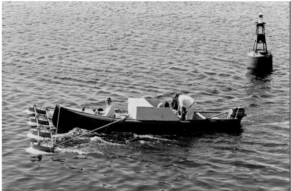
*Fig. 3 Raytheon 719 Channel Sweep System using a boom system developed by the Canadian Hydrographic Service.*
