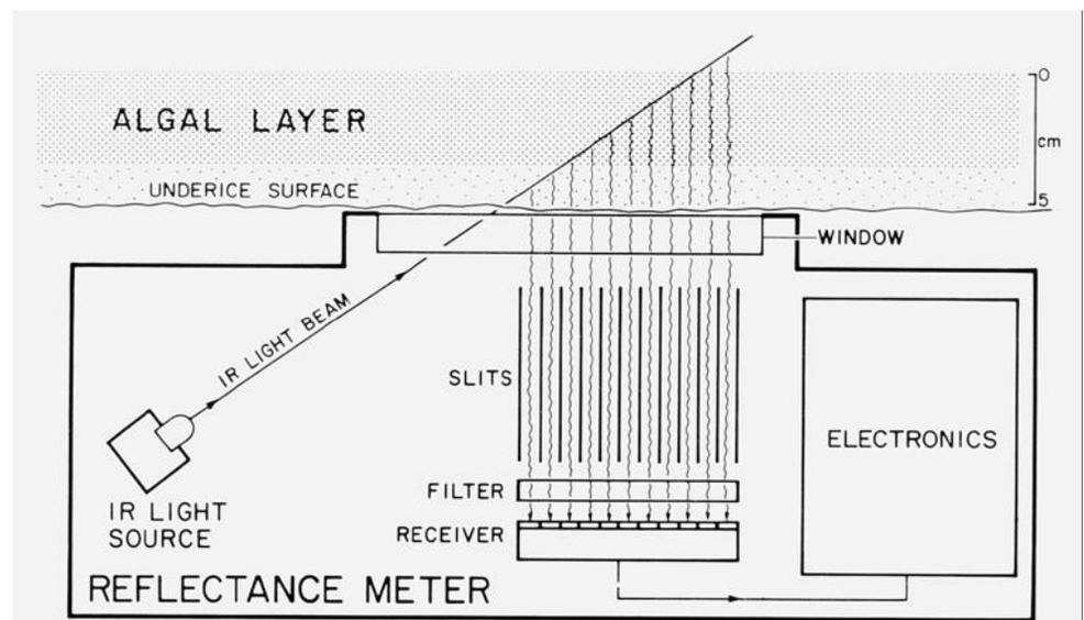
Fig. 3 The reflectance meter used to detect algal layers in the underice surface.
