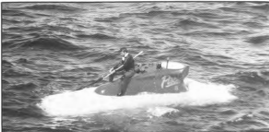
The PISCES submersible is a piloted mini-submarine capable of taking two observers more than 1000 metres (3000 ft.) beneath the ocean's surface. Here it is being used to find capelin spawn on the Southeast Shoal.
