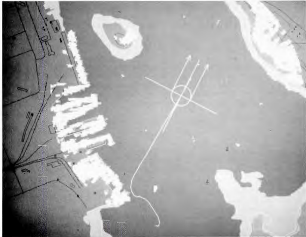
Electronic Chart Testbed display in Halifax Harbour at 1:10 000. Note the smooth tracking by NAVSTAR GPS, which plots the ship (and hence the radar) about 30 metres east in relation to the coastline on this North American datum chart. The datum shift is about to be removed using the "positioner offset." The ship's guard circle is set to 0.5 cables (100 m) and the parallel index bars show course made good, which at present coincides with small ship's-head pointer on the centre line. (NOTE: On the colour video, the light blue shoal water is clearly distinguished from the light olive land; this disappears in black and white reproduction.)
