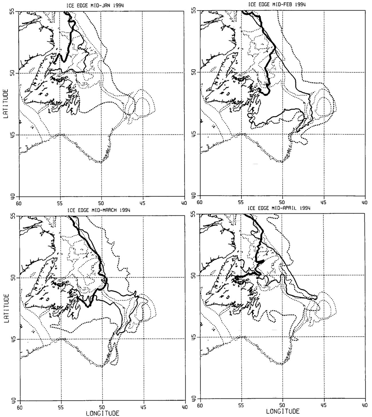
Fig. 2a. Ice edge locations for mid-January to mid-April of 1994 (light solid lines). The dashed and heavy solid lines are locations for the maximum and median positions for the same time period based on historical data from 1962 to 1987. (from Cote, 1989)
