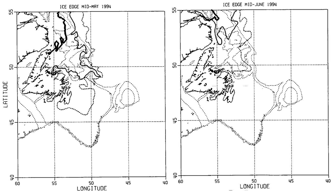
Fig. 2b. Ice edge locations for mid-May and mid-June of 1994 (light solid lines). The dashed and heavy solid lines are locations for the maximum and median positions for the same time period based on historical data from 1962 to 1987. (from Cote, 1989)
