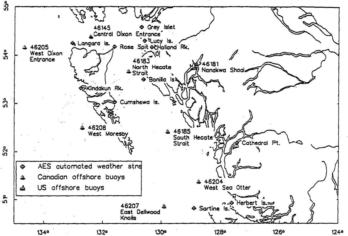
**Figure 14a. Meteorological buoys and automated meteorological stations - North coast.**
