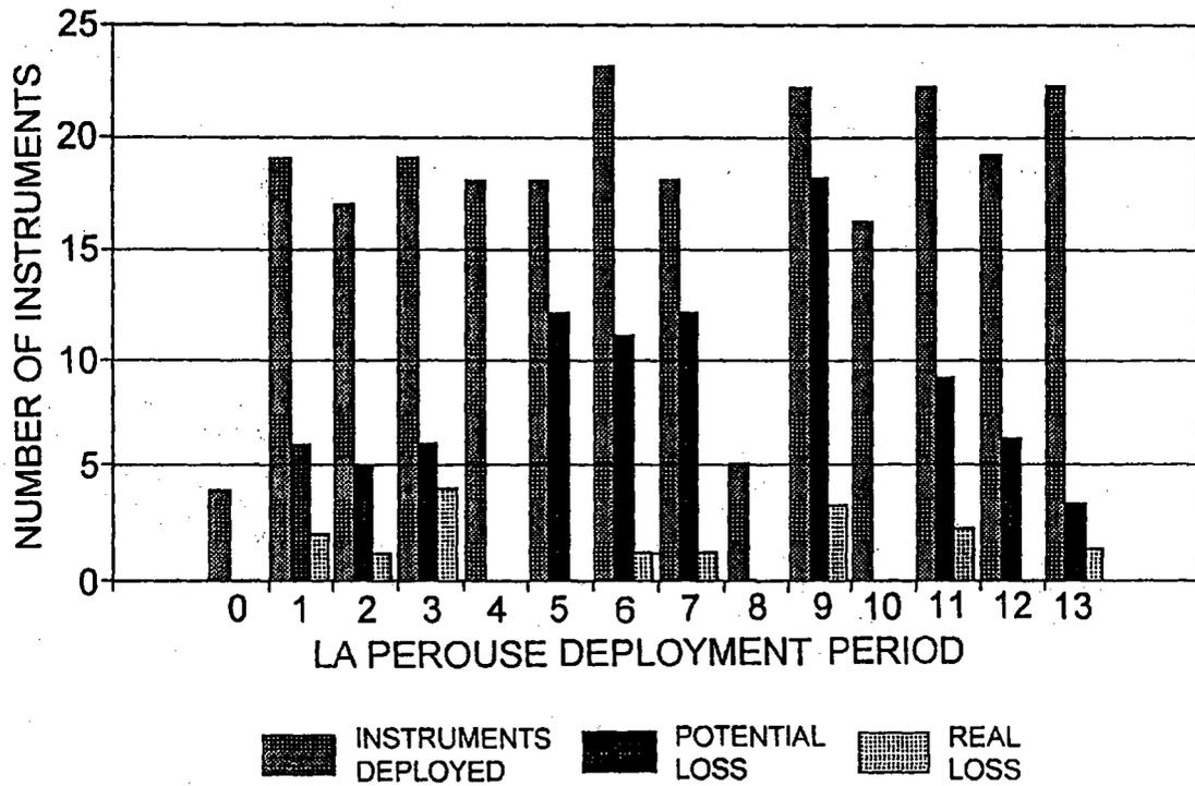
Figure 5. Summary of La Perouse mooring losses for the period November 1984 to October 1991. Bar graph shows total number of current meters, pressure gauges and transmissometers deployed during each field servicing period, the number of instruments (potential loss) that were damaged, failed to be recovered through normal operations or went adrift, and the actual (real) loss of instruments.
