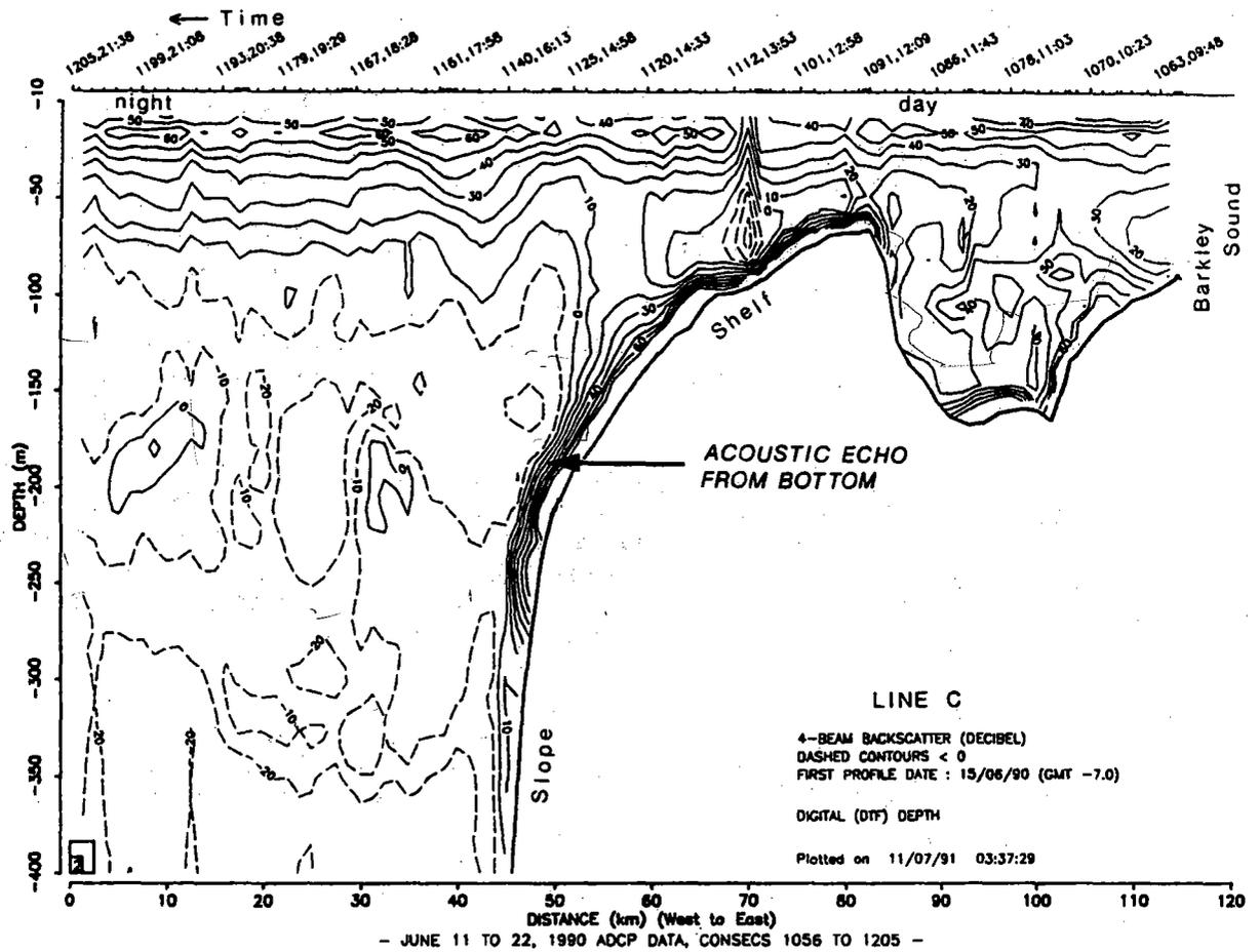
Figure 8. Cross-section of four-beam averaged backscatter intensity (in decibels) taken on June 15, 1990 along Line C using the shipboard 150 kHz acoustic Doppler profiler on the CSS Parizeau. Each profile (tick mark) is based on a 5-minute average. The header gives the ensemble number (1055-1205) and local time (PDT). The large intensities near the bottom result from side-lobe backscatter from the seafloor; values within 15% of the bottom are not reliable.
