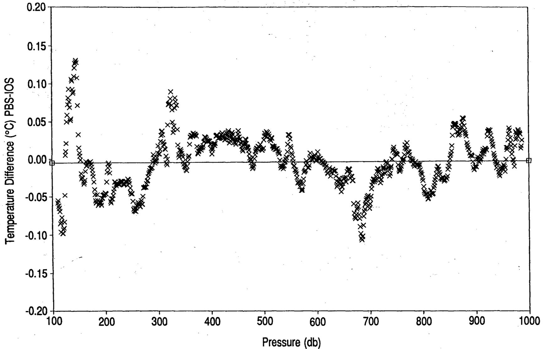
Figure 9a. Inter-comparison of temperature data collected from the PBS and IOS Guildline CTD systems on July 23, 1991 at 49°28.7'N; 127°20.7'W (diff = PB-IOS). Only values for depths greater than 100 decibars (about 100 m) are shown. The least squares linear fit to the data is displayed.
