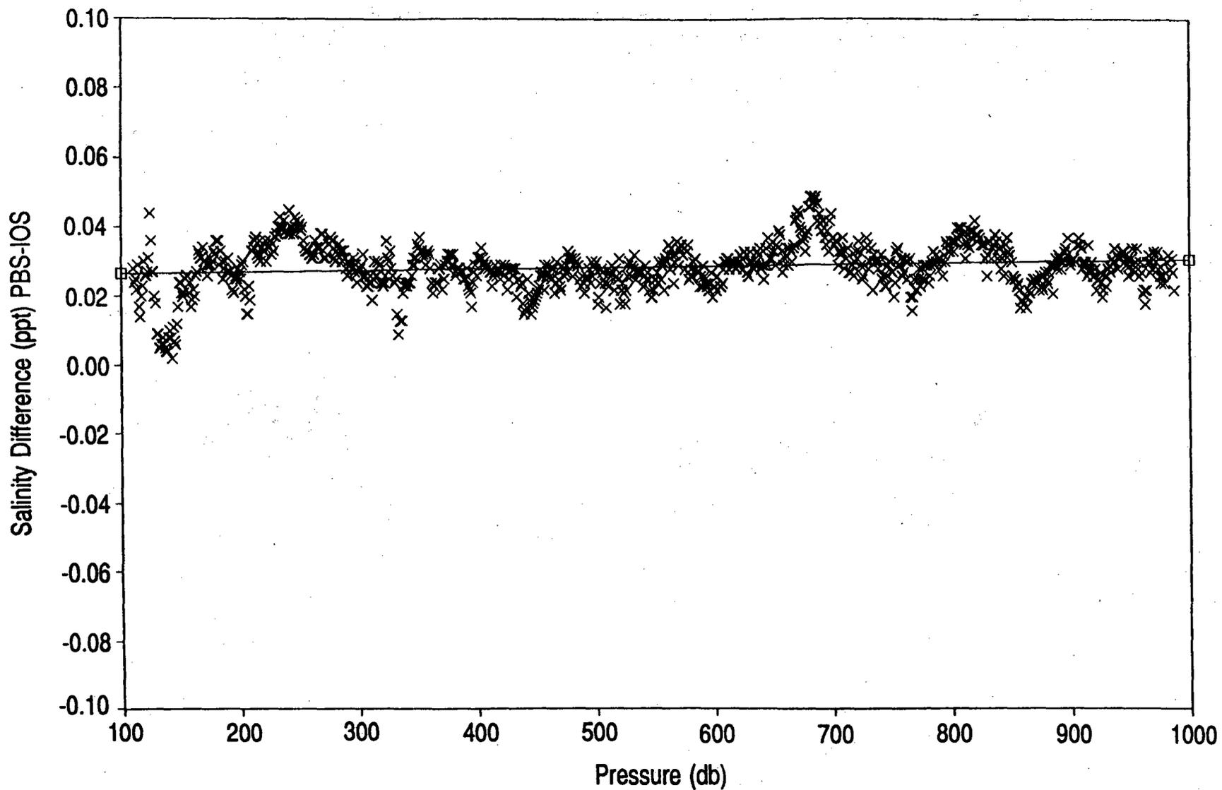
Figure 9b. Inter-comparison of salinity data collected from the PBS and IOS Guildline CTD systems on July 23, 1991 at 49°28.7'N; 127°20.7'W (diff - PBS-IOS). Only values for depths greater than 100 decibars (about 100 m) are shown. The least squares linear fit to the data is displayed.
