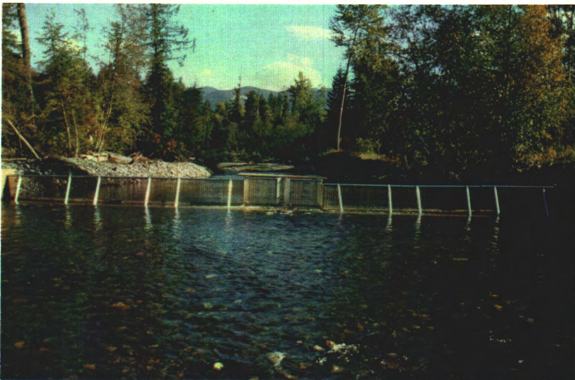
Photo 2.4 Enumeration fence on Louis Creek (photo courtesy of M. Sheng)
