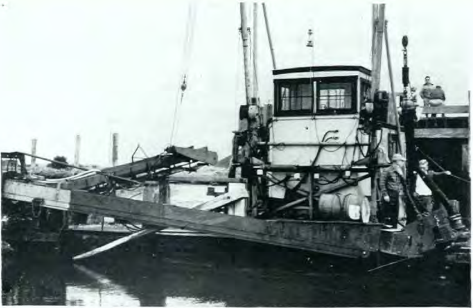
FIG. 84. Escalator-type oyster harvester.
