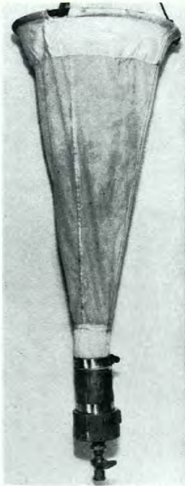
FIG. 55. Plankton net used in sampling oyster larvae. \times 0.2 .
