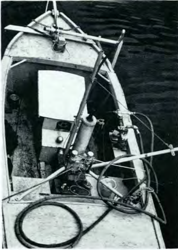
FIG. 57. Pipe sampler for oyster larvae mounted on the starboard bow of a launch. The pipe leads back to a water meter and to the motor-powered pump; the long marked hose is used for taking spot samples from various depths.
