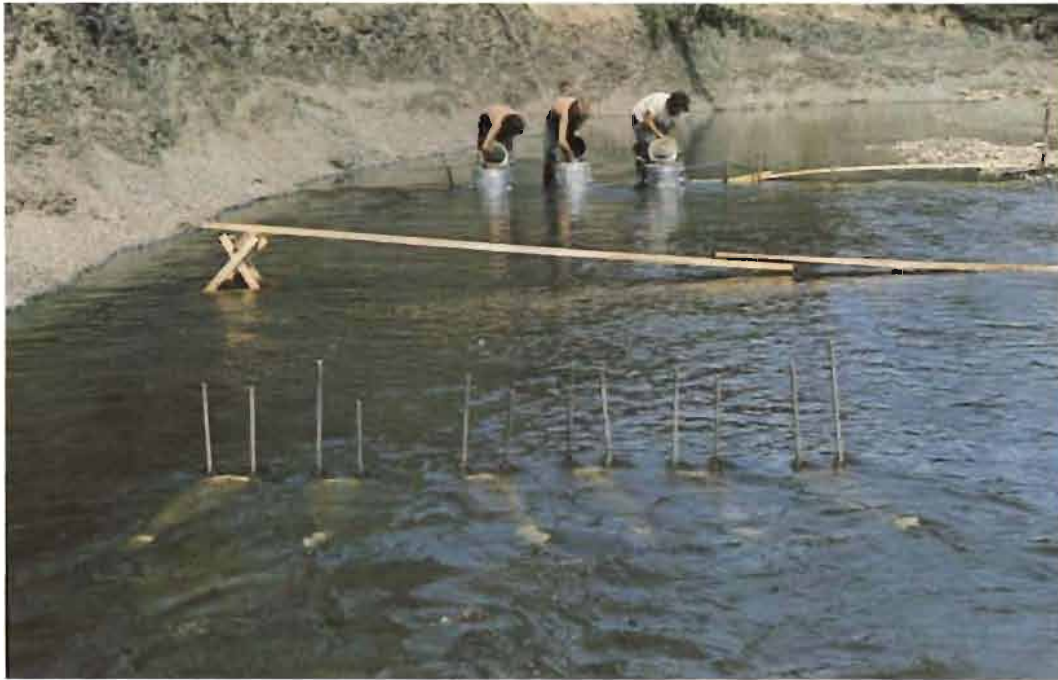
Figure 12. Sediment dispensers used in the Harris River sediment addition experiments: (a) for high discharge periods; (b) for low discharge periods. Water flow is toward the viewer. Note cutback, from which sediment was obtained, to the side. Sediment dispensers and plank from which sediment slurry was poured are at the top of the channel. Water samples for suspended sediment analysis at 7.5 m were taken off the plank at mid-channel. Driftnets are at the lower end of the channel.
