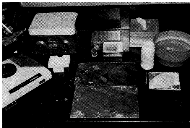
FIG. 10. Typical polishing workstation. From left to right: Olympus compound microscope with high intensity light attachment; hot-plate kept at 40–60°C; box of cut pieces of glass for the second polish; polishing board with 220, 400, and 600 grit sandpaper; thermoplastic glue; tissue well tray for otolith storage; box of glass slides; Kimwipes; polishing slurry (water and 0.3 µm alumina); polishing cloth; bowl of water.
