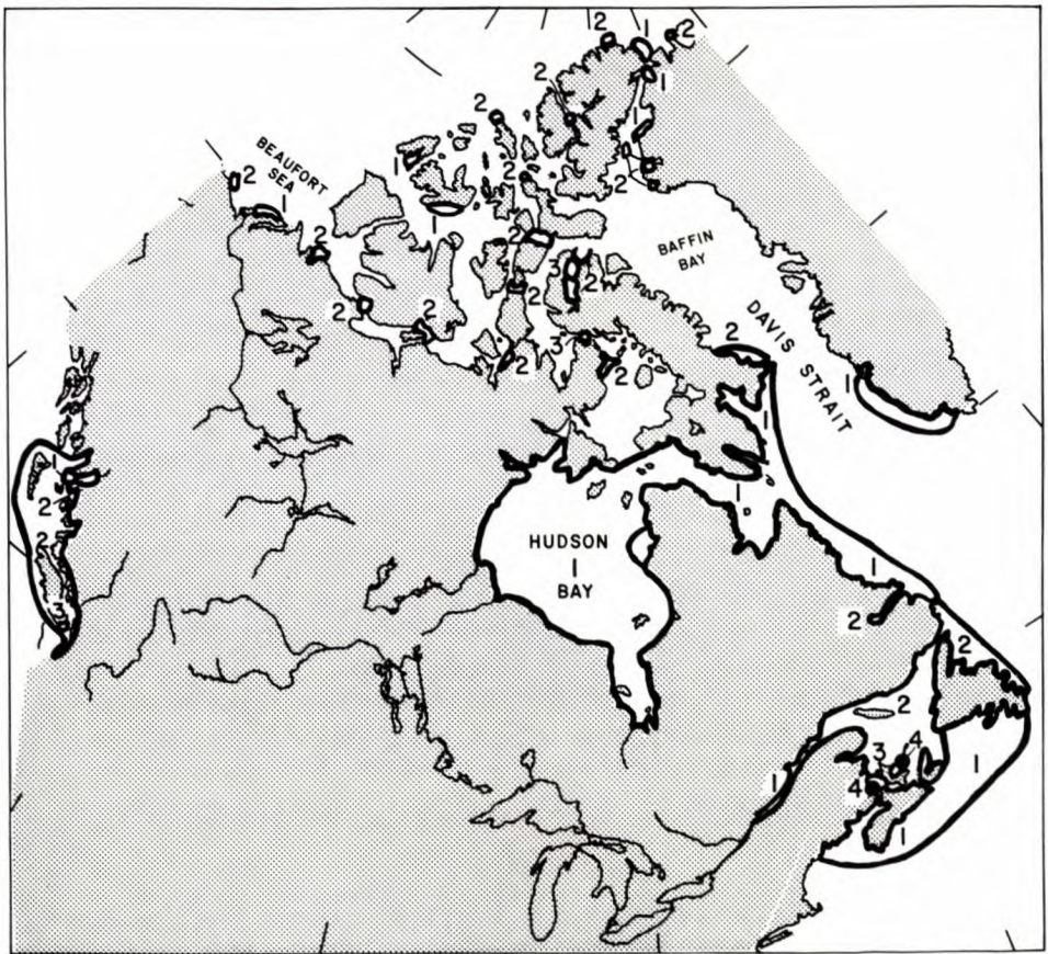
FIG. 5.16. Tides in Canadian waters classified according to the following scheme: 1, semidiurnal; 2, mixed, mainly semidiurnal; 3, mixed, mainly diurnal; 4, diurnal. (Dohler 1967b)
