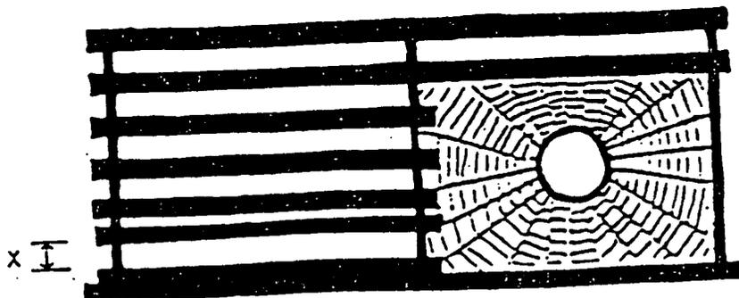
Figure 4 - Diagram of a lobster trap used in the Salmon Beach or Miminegash study where the wooden lath space, X, is varied to 34.9, 37.1, 38.1 or 44.4 mm.
