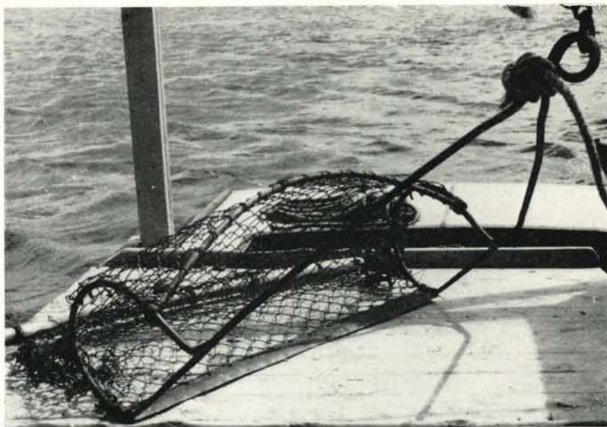
FIG. 40. Oyster dredge (blade 30 inches) aboard the Royal II (Victor Travers, owner) which is typical of larger oyster boats of southern Malpeque Bay, P.E.I. The dumping ring at the centre of the club stick does not show clearly through the flexible-mesh wire bag.
