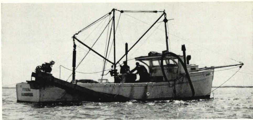
FIG. 42. Escalator harvester modified by Fisheries Research Board for fishing oysters. Water is fed from an inboard pump through 4-inch hose to the scoop which is submerged. (Photo: R. E. Drinnan.)
