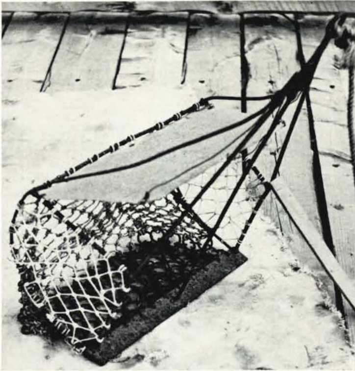
FIG. 38. Small oyster dredge (blade 18 inches) commonly used from outboard motor boats in Bideford River, P.E.I. The pressure plate permits light construction for easier manual hoisting. The angle of the plate can be changed by adjusting the length of the wires joining its forward corners to the frame.
