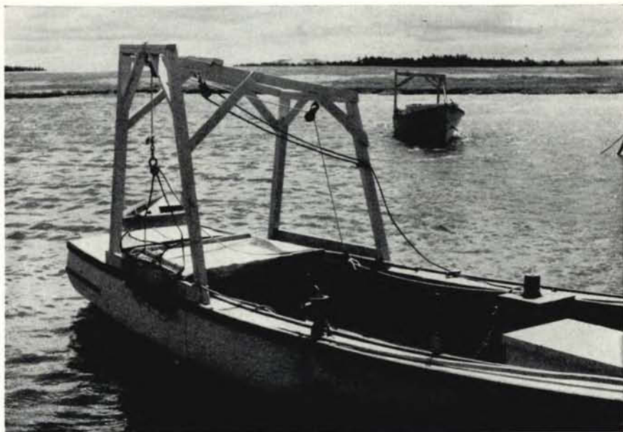
FIG. 41. Stern gallows, culling table and rigging for towing dredge from the starboard quarter of Royal II . The tow line lies slack across the culling table but the hoisting line is taut and leads through three blocks to the niggerhead on the right. The dumping line with its hook is looped over a nail in the forward upright on the port side to keep it out of the way when not in use. It leads through two blocks, one on the gallows and one on the gunwale.
