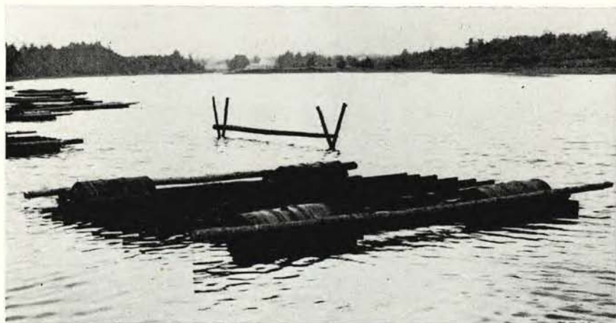
FIG. 19. Gasoline drum float for suspending collectors.
