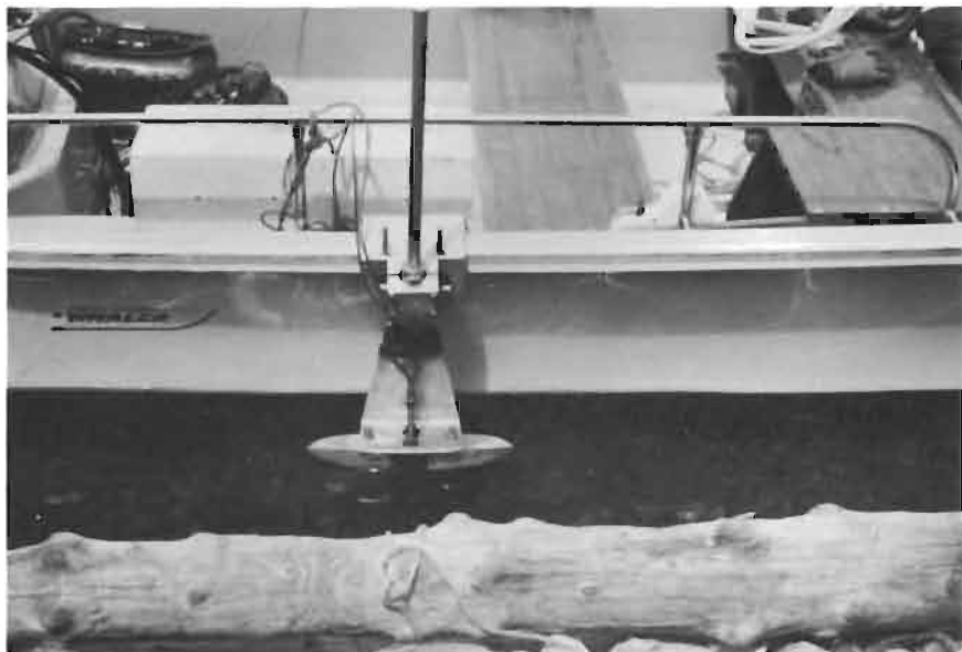
Figure 18. Outrigger-type transducer arm with transducer mounted on the gunwale of a Boston Whaler.
