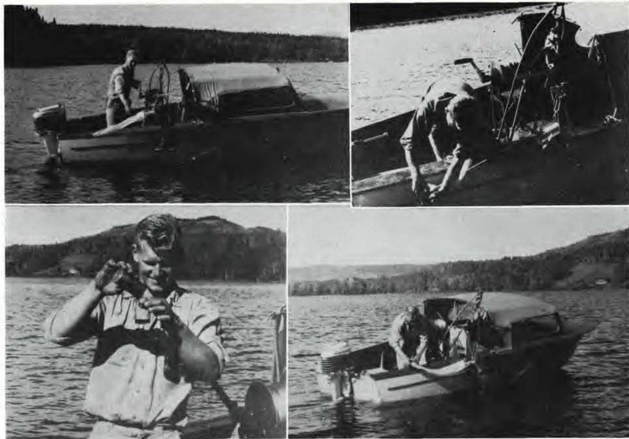
PLATE IX. Clarke-Bumpus plankton sampler in operation.
